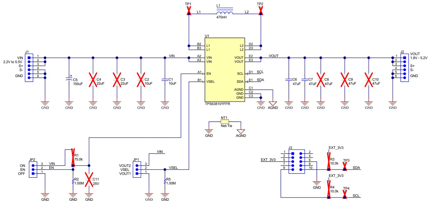
Figure 7. TPS6381xEVM Schematic
