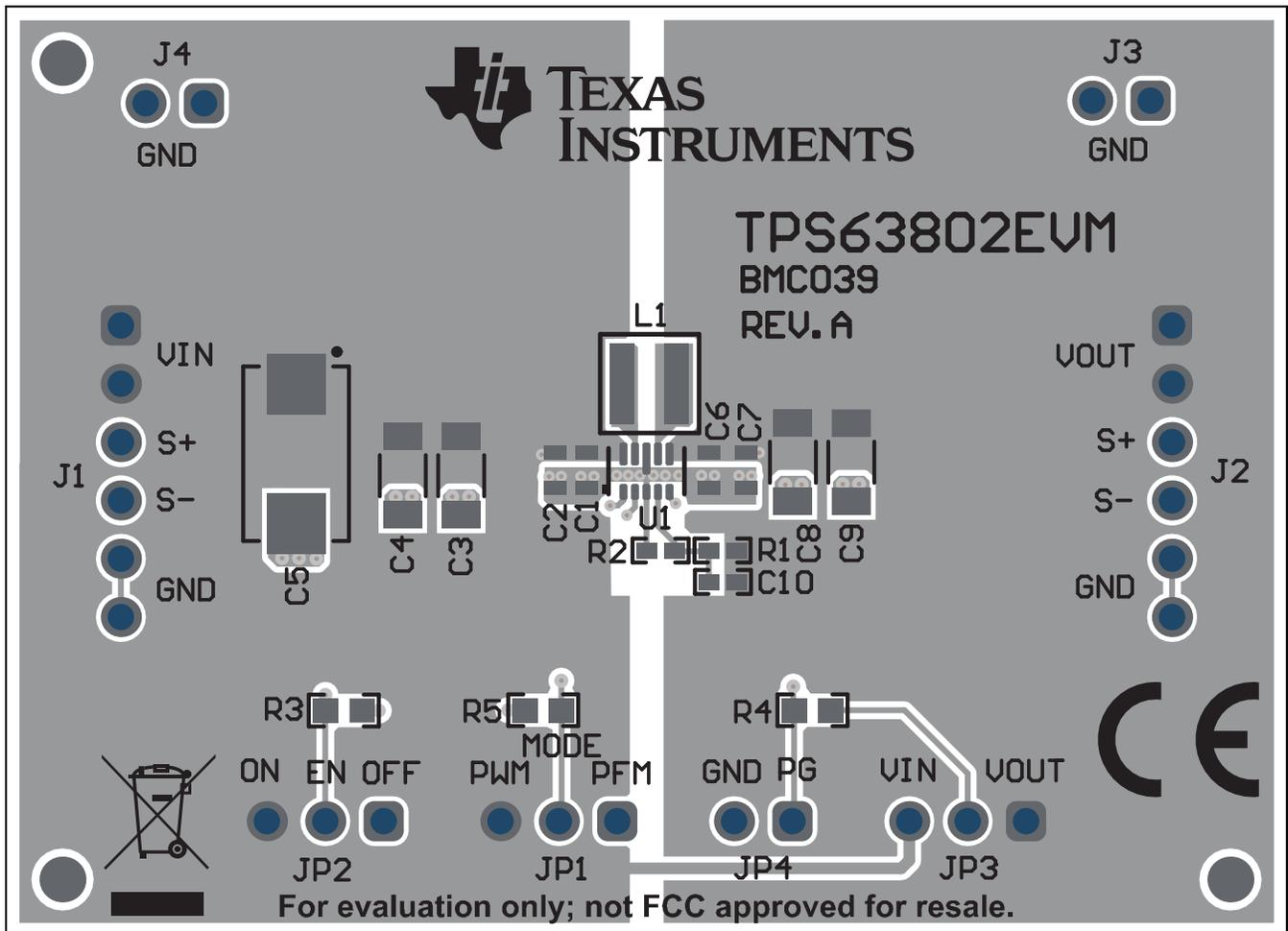
Figure 2. Assembly Layer
