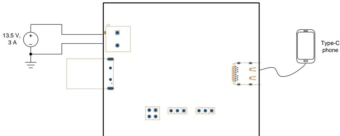
**Figure 2. EVM Setup for Charging USB Type-C™ Device**
