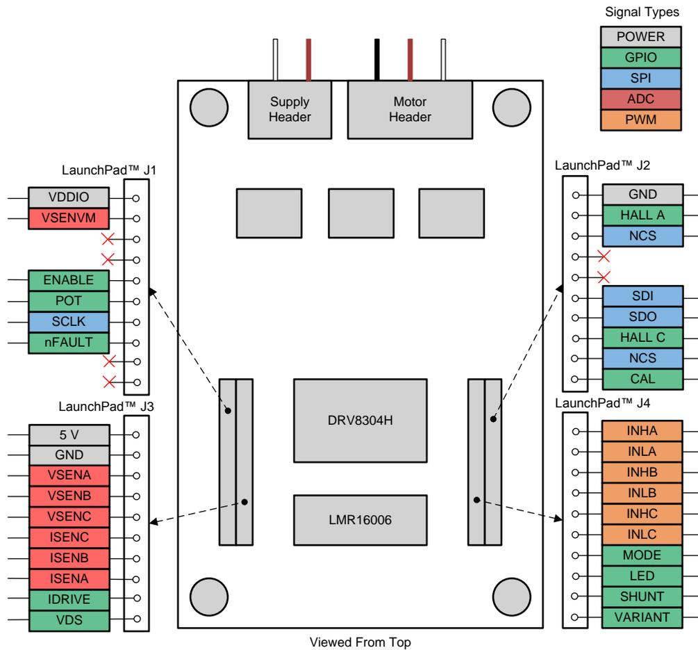
Figure 4. BOOSTXL-DRV8304H Jumper Connectors Pinout
