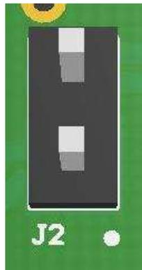
Figure 12. Potentiometer Power Header (J2)
