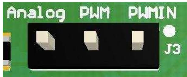
Figure 11. Speed Command Input Select Header (J3)
