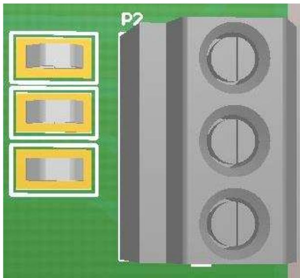
Figure 6. Motor Phase Windings Input Terminal Block (P2)
