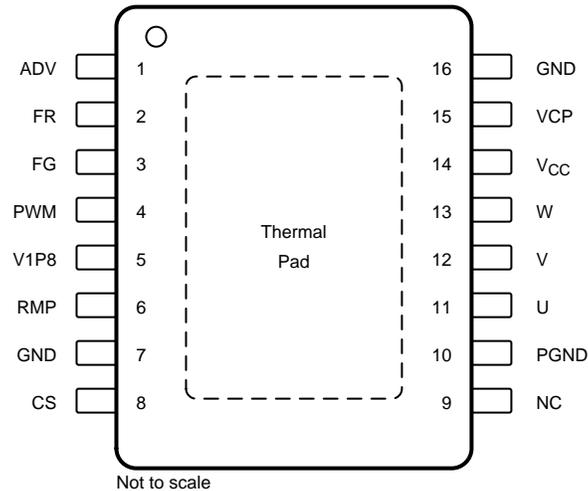
**Figure 7. DRV10974PWP Pinout**
