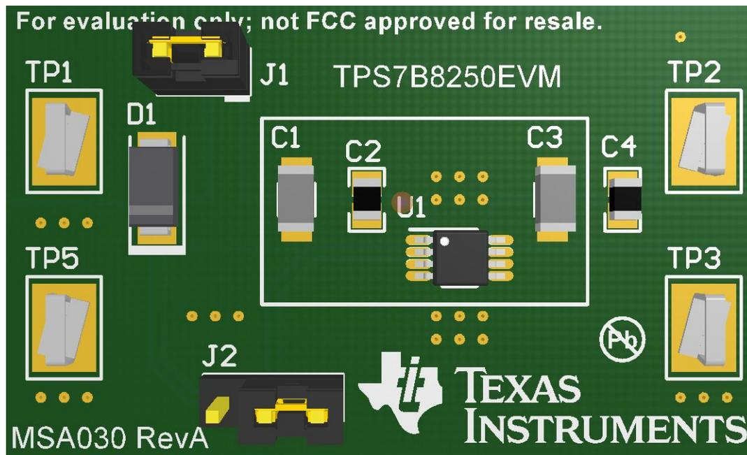
This user's guide describes operational use of the TPS7B8250 evaluation module (EVM) as a reference design for engineering demonstration and evaluation of the TPS7B82-Q1 low-dropout (LDO) linear regulator. Included in this user's guide are setup instructions, a schematic diagram, printed circuit board (PCB) layout, and a bill of materials (BOM).
