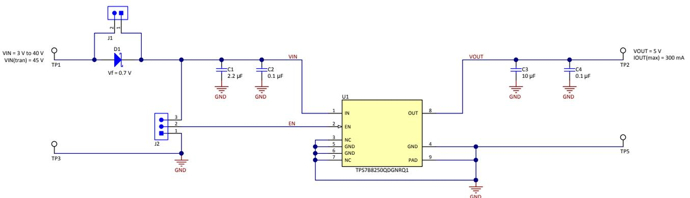
Figure 1. TPS7B8250EVM Schematic
