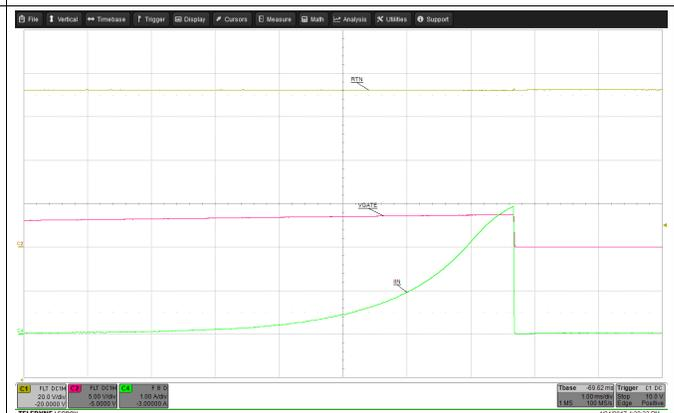
Figure 7. Start-into-Short Zoomed in ( $V_{IN} = 72\text{ V}$ )
