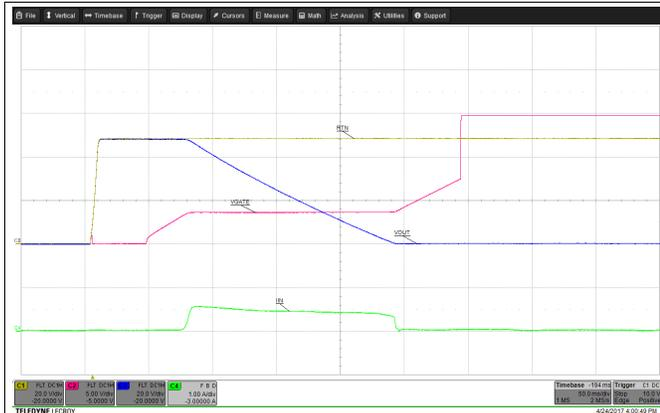
Figure 2. Start-up ( $V_{IN} = 48\text{ V}$ ,  $C_{OUT} = 1.32\text{ mF}$ )
