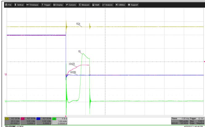
Figure 8. Hot-Short With No Load ( $V_{IN} = 72\text{ V}$ )
