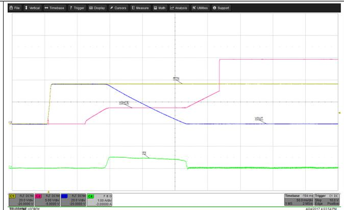
Figure 3. Start-up ( $V_{IN} = 36\text{ V}$ ,  $C_{OUT} = 1.32\text{ mF}$ )
