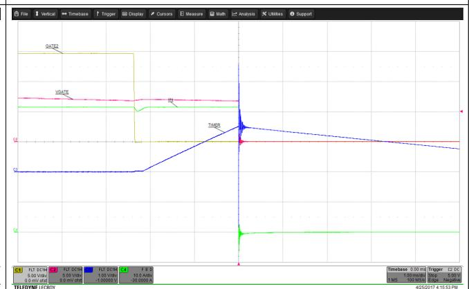
Figure 11. Gradual Overcurrent ( $V_{IN} = 36\text{ V}$ )
