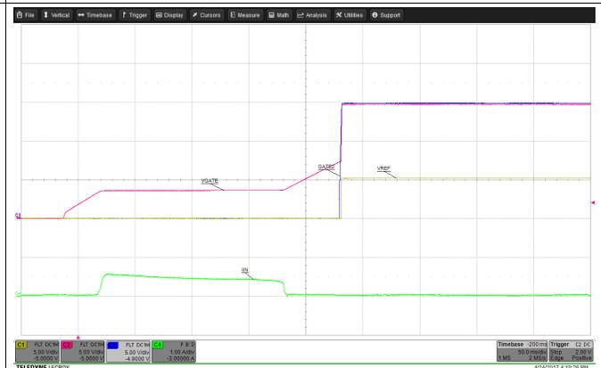
Figure 5. Start-up Showing VREF and GATE2
