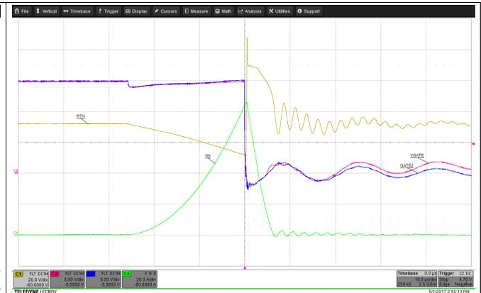
Figure 9. Hot-Short With no Load Zoomed In ( $V_{IN} = 72\text{ V}$ )
