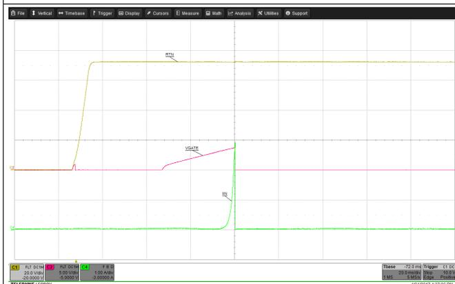
Figure 6. Start-into-Short ( $V_{IN} = 72\text{ V}$ )
