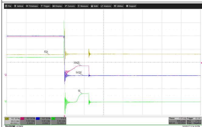
Figure 10. Hot-Short With 1.2-kW Load ( $V_{IN} = 72\text{ V}$ )
