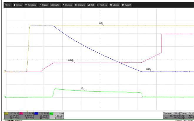
Figure 4. Start-up ( $V_{IN} = 72\text{ V}$ ,  $C_{OUT} = 1.32\text{ mF}$ )
