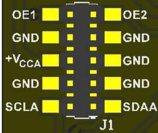
J1 is the connector designed to be mated with any I<sup>2</sup>C master via 0.100" headers. J1 allows for power connection (+V<sub>CCA</sub>), ground connection, OE1 for U1, OE2 for U2, SDA, and SCL data lines. U2 is by default loaded with TCA9802. Connect +V<sub>CCA</sub> to the EVM using J1-6.
