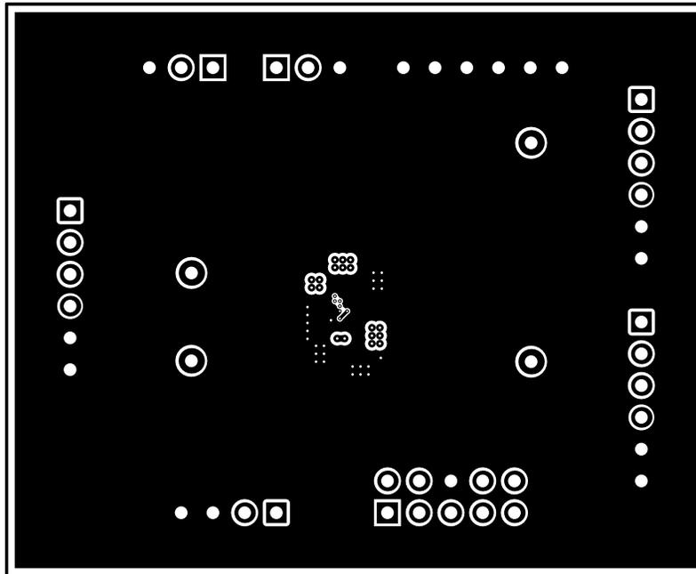
Figure 17. PCB Inner Layer 1 (Top View)
