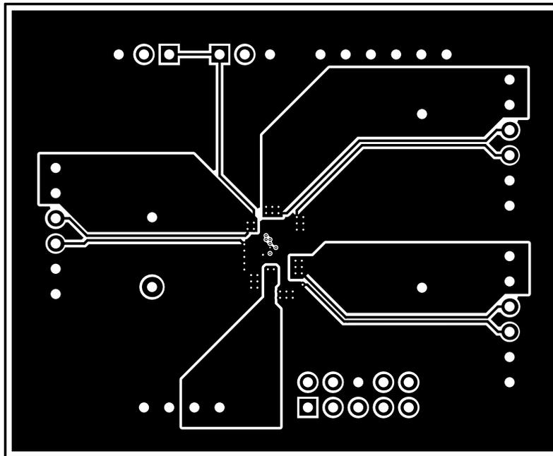
Figure 18. PCB Inner Layer 2 (Top View)
