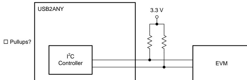
**Figure 12. I<sup>2</sup>C Bus External Pullup Connection**
