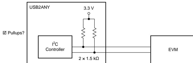
**Figure 11. I<sup>2</sup>C Bus Internal Pullup Connection**
