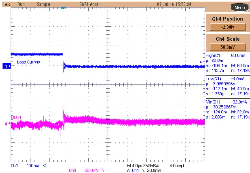
Figure 17. PFM Load Transient Response: VOUT1 Falling Edge
