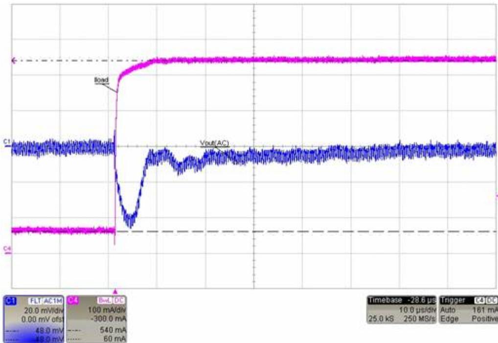
Figure 14. PWM Load Transient Response: VOUT2 Rising Edge
