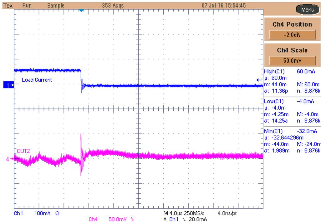
Figure 19. PFM Load Transient Response: VOUT2 Falling Edge
