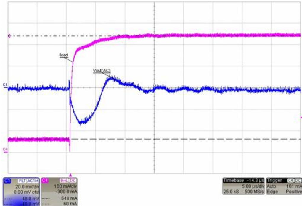
Figure 12. PWM Load Transient Response: VOUT1 Rising Edge
