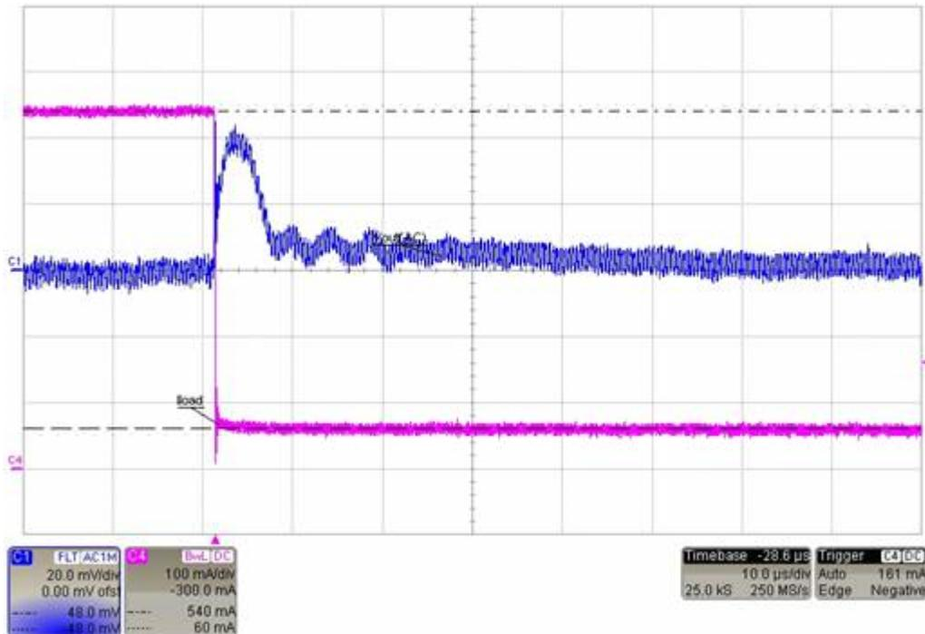
Figure 15. PWM Load Transient Response: VOUT2 Falling Edge
