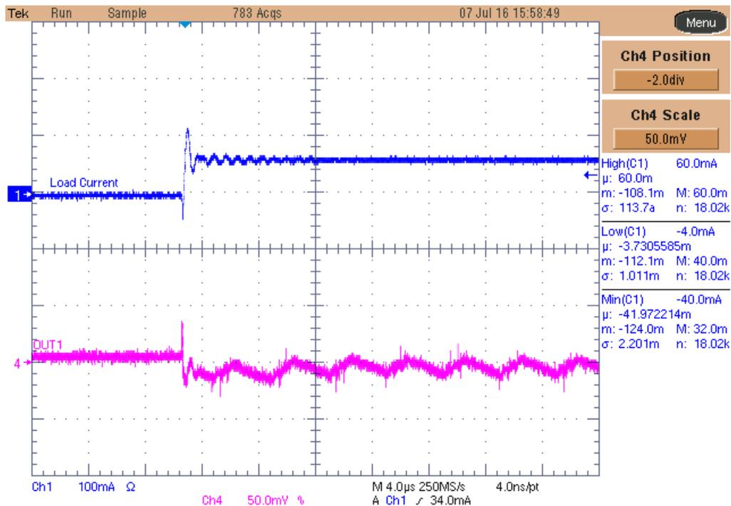
Figure 16. PFM Load Transient Response: VOUT1 Rising Edge
