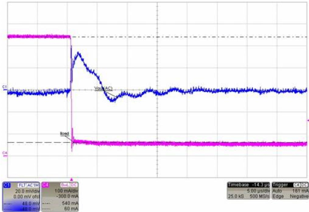
Figure 13. PWM Load Transient Response: VOUT1 Falling Edge
