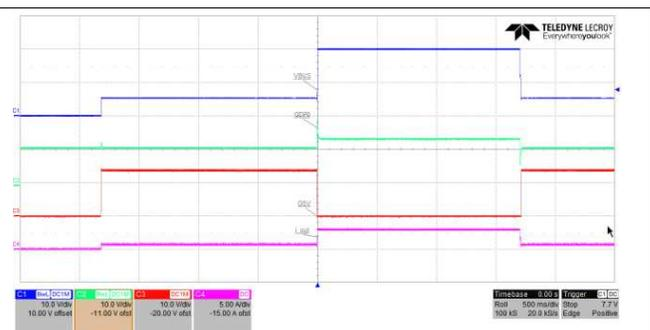
Figure 9. Mux Between 5 V and 20 V at 3 A
