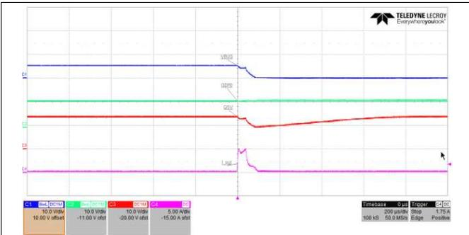
Figure 18. 5.5-A Load Step Triggers OCP (5 V)
