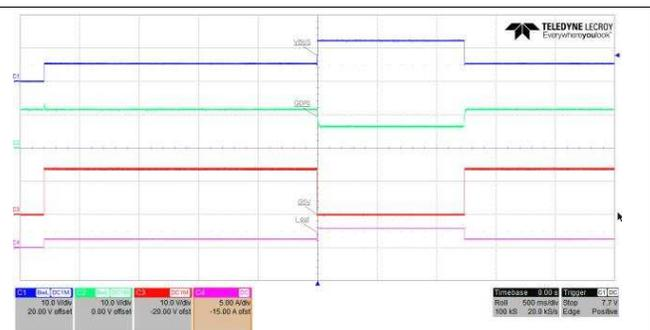
Figure 7. Mux Between 5 V and 12 V at 3 A
