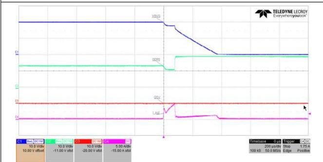
Figure 20. 5.5-A Load Step Triggers OCP (20 V)
