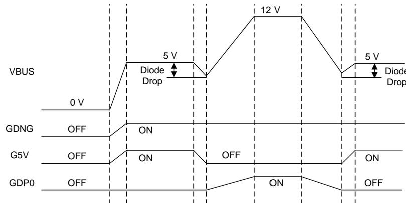
**Figure 2. Switching Between 5 V and 12 V Using GDNG, G5V, and GDPG**
