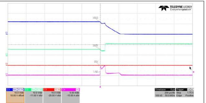
Figure 19. 5.5-A Load Step Triggers OCP (12 V)
