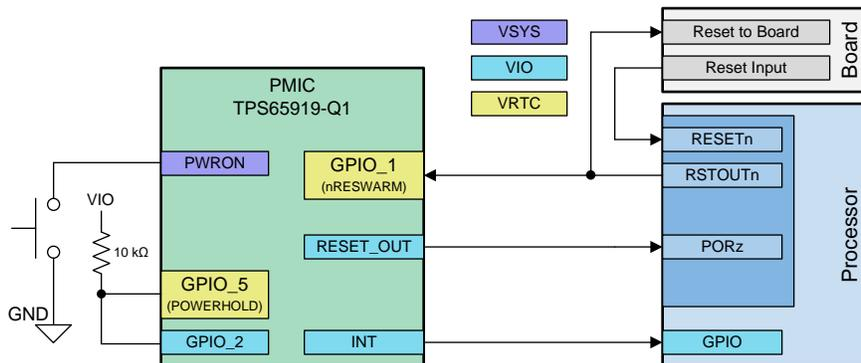
**Figure 4. Reset Connections With PWRON Configuration**
