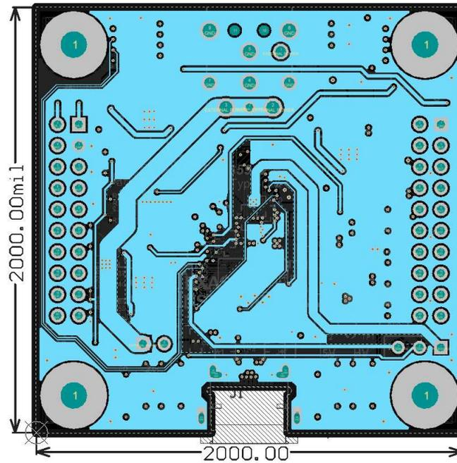
Figure 10. PCB Layer 5 (Inner Signal Layer 2)
