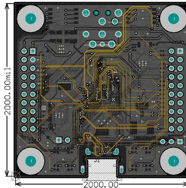
Figure 8. PCB Layer 3 (Inner Signal Layer 1)
