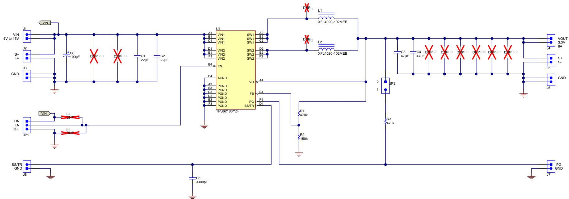
Figure 9. TPS62180EVM-581 Schematic
