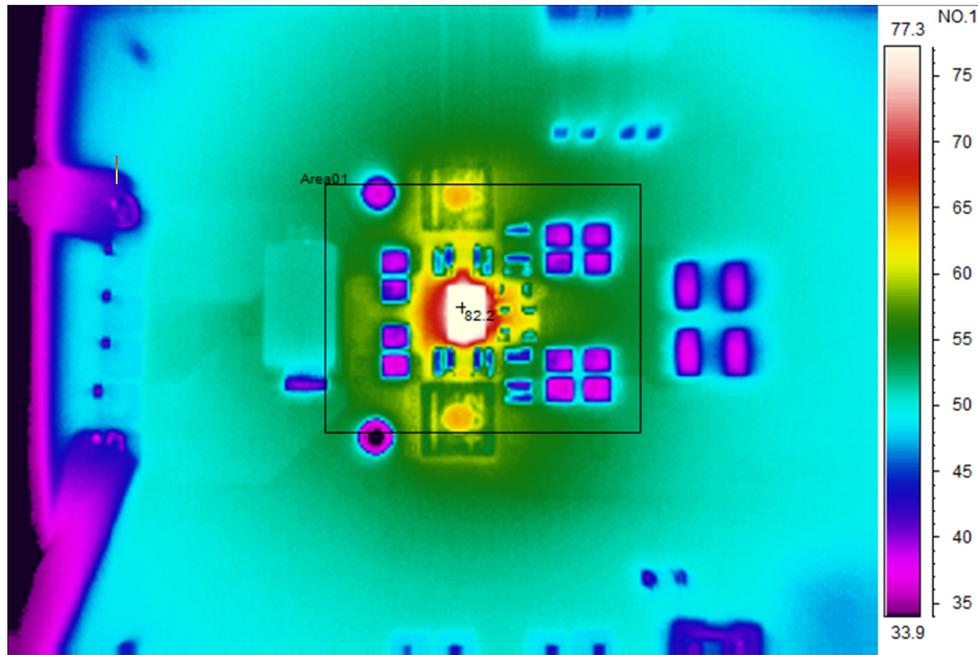
Figure 1. Thermal Performance ( $V_{IN} = 15\text{ V}$ , Load = 6 A)
