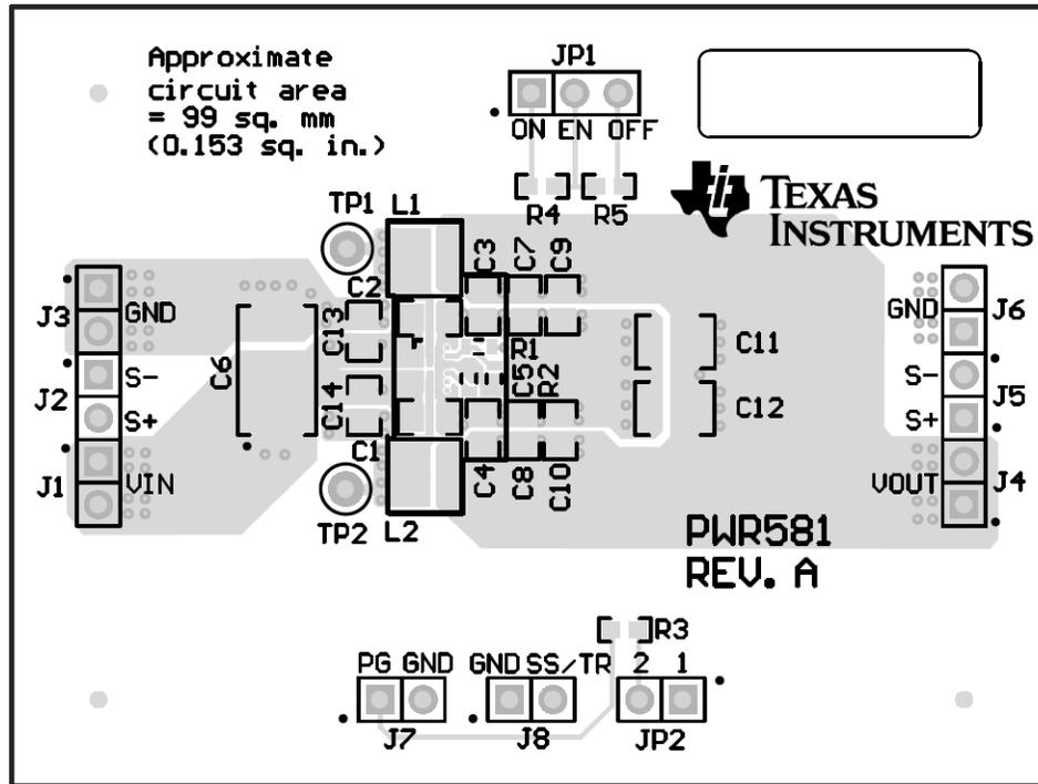
Figure 3. Assembly Layer
