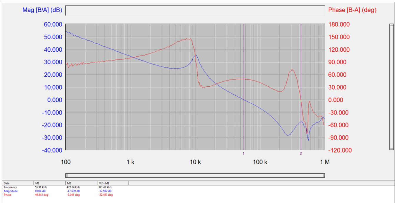
Figure 11. Bode Plot (12 V<sub>IN</sub>, 1.2 V<sub>OUT</sub>, 20 A)
