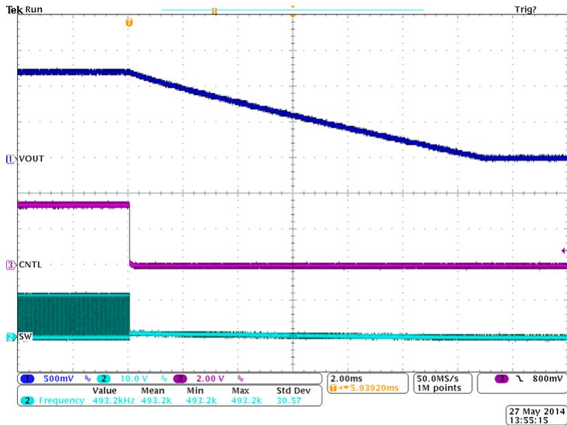
Ch1 =  $V_{OUT1}$  at 500 mV/division, Ch2 = SW node at 10 V/division, Ch3 = CNTL1 at 2 V/division
