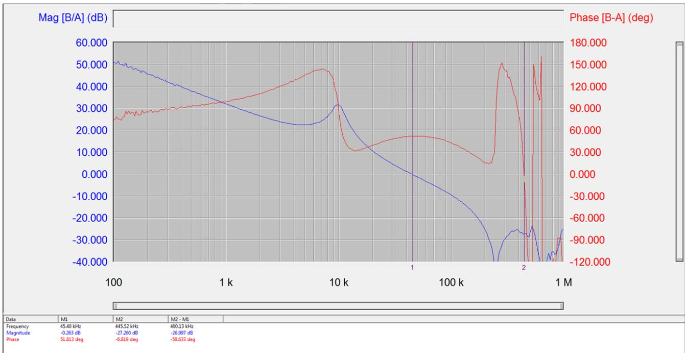
Figure 12. Bode Plot (12 V<sub>IN</sub>, 1.8 V<sub>OUT</sub>, 20 A)
