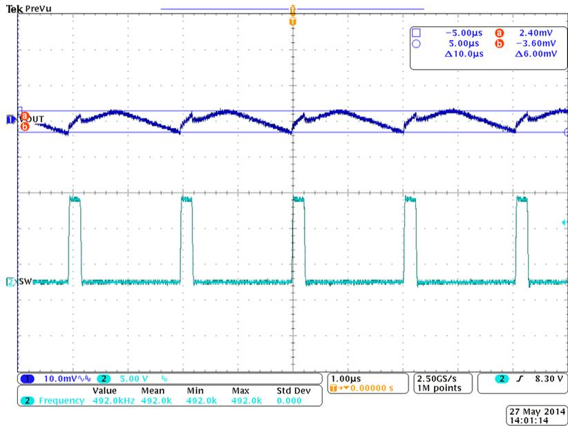
Ch1 =  $V_{OUT1}$  at 10 mV/division, Ch2 = SW node at 5 V/division
