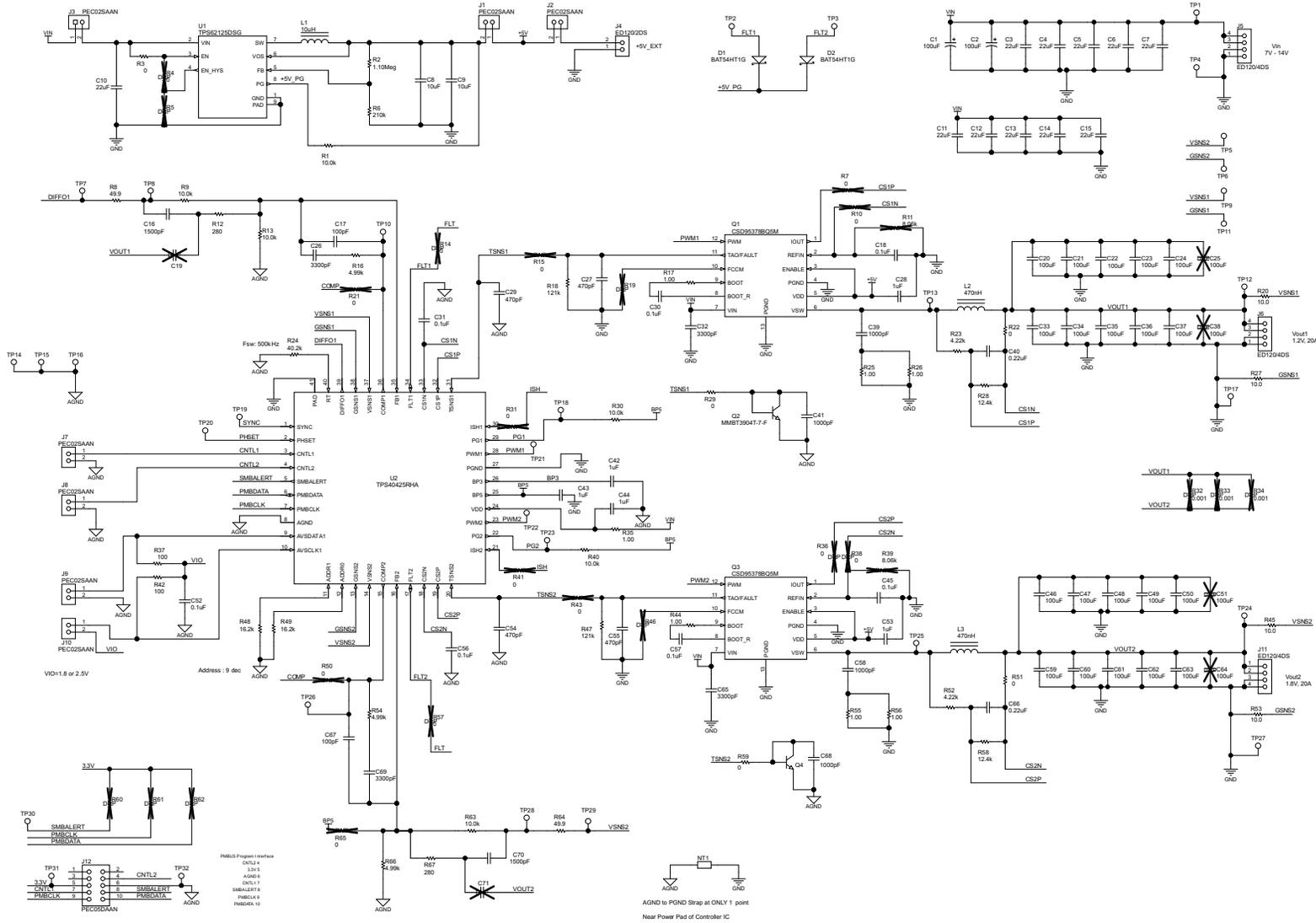
Figure 1. TPS40425EVM-PWR594 Schematic
