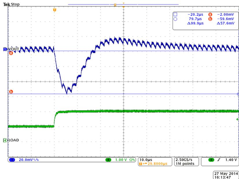
Ch1 =  $V_{OUT2}$  at 20 mV/division, Ch2 =  $I_{OUT2}$  at 10 A/division
