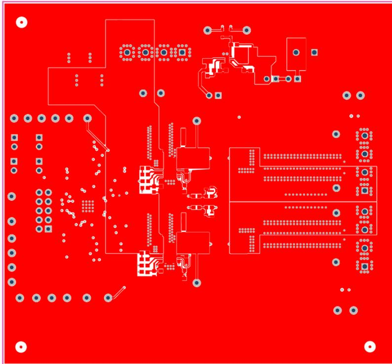
Figure 25. PWR594 EVM Top Copper (Top View)
