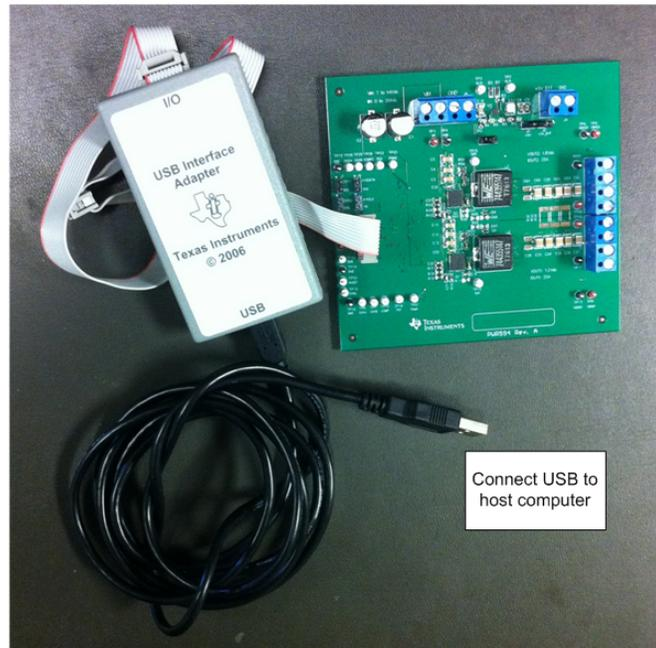
**Figure 4. Texas Instruments USB-to-GPIO Adapter and Connections**
