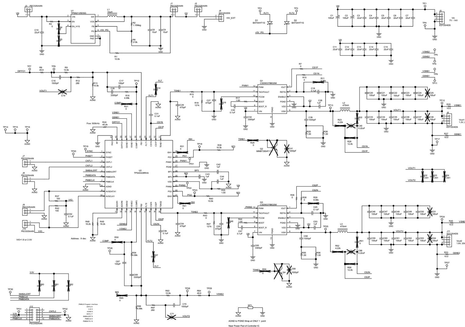
Figure 2. TPS40428EVM-PWR594 Schematic
