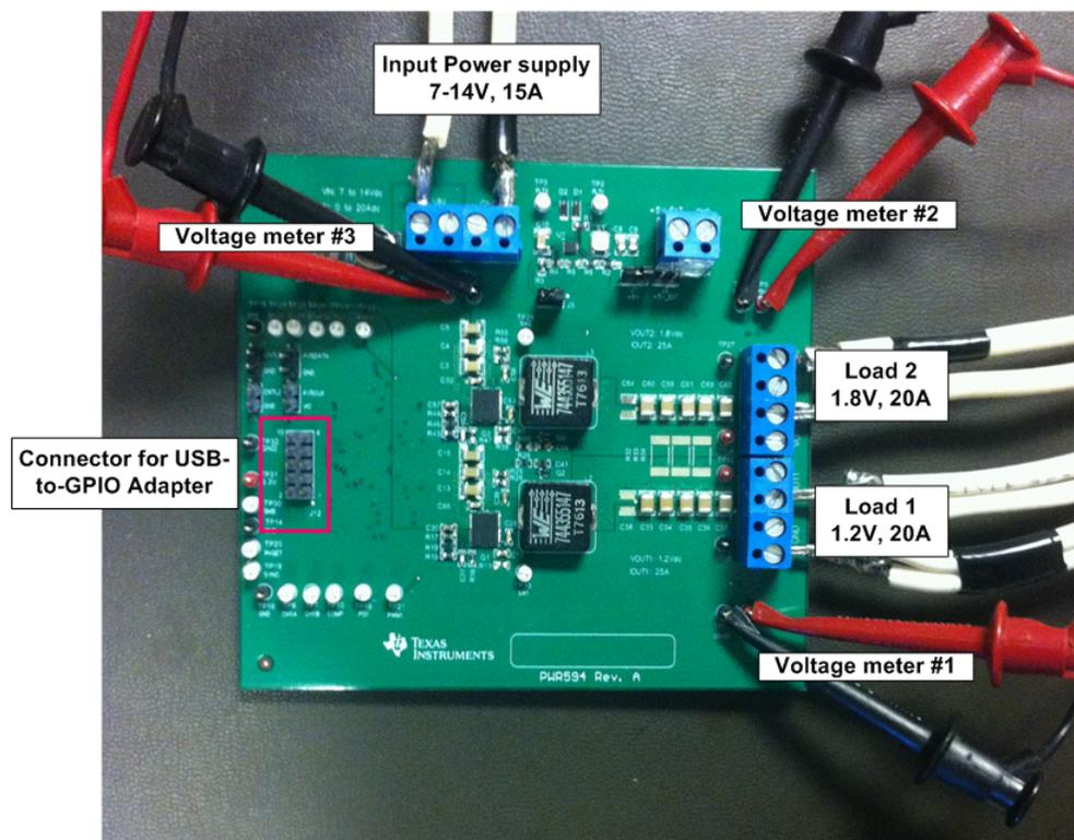
Figure 3. PWR594 EVM Recommended Test Set Up
