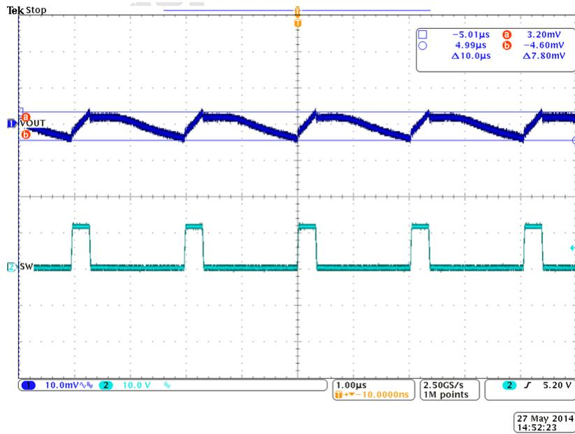
Ch1 =  $V_{OUT2}$  at 10 mV/division, Ch2 = SW node at 10 V/division
