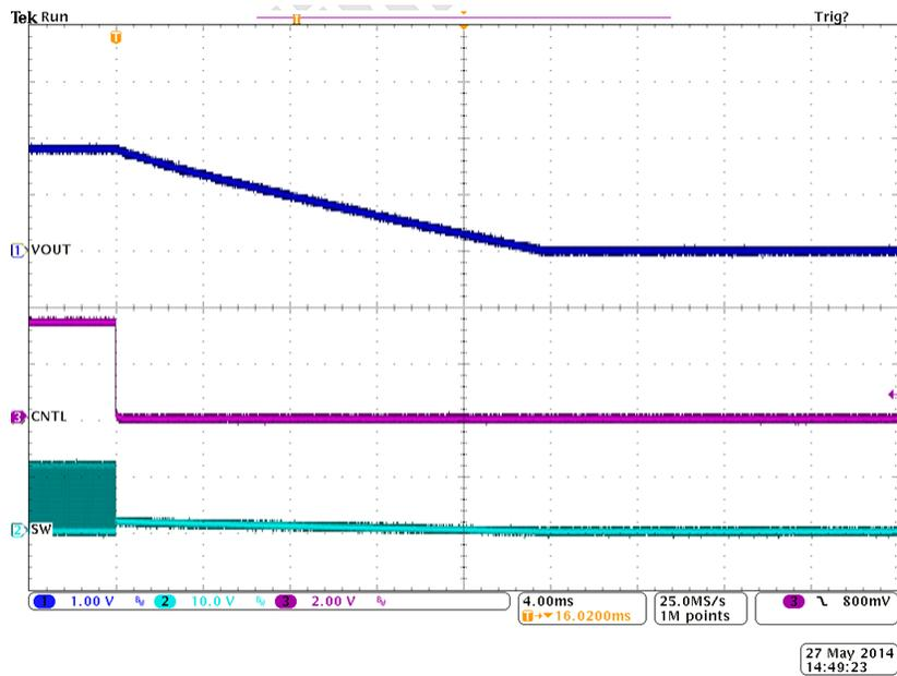
Ch1 =  $V_{OUT2}$  at 1 V/division, Ch2 = SW node at 10 V/division, Ch3 = CNTL2 at 2 V/division
