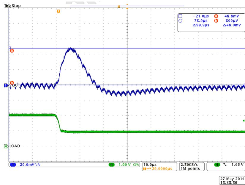
Ch1 =  $V_{OUT1}$  at 20 mV/division, Ch2 =  $I_{out1}$  at 10 A/division
