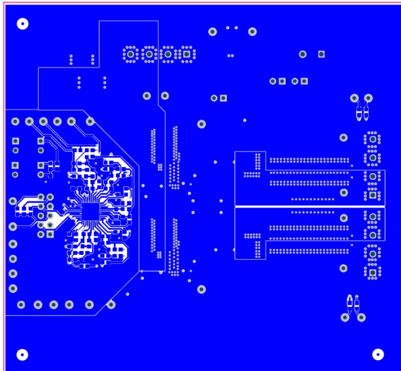
Figure 30. PWR594 EVM Bottom Copper (Top View)
