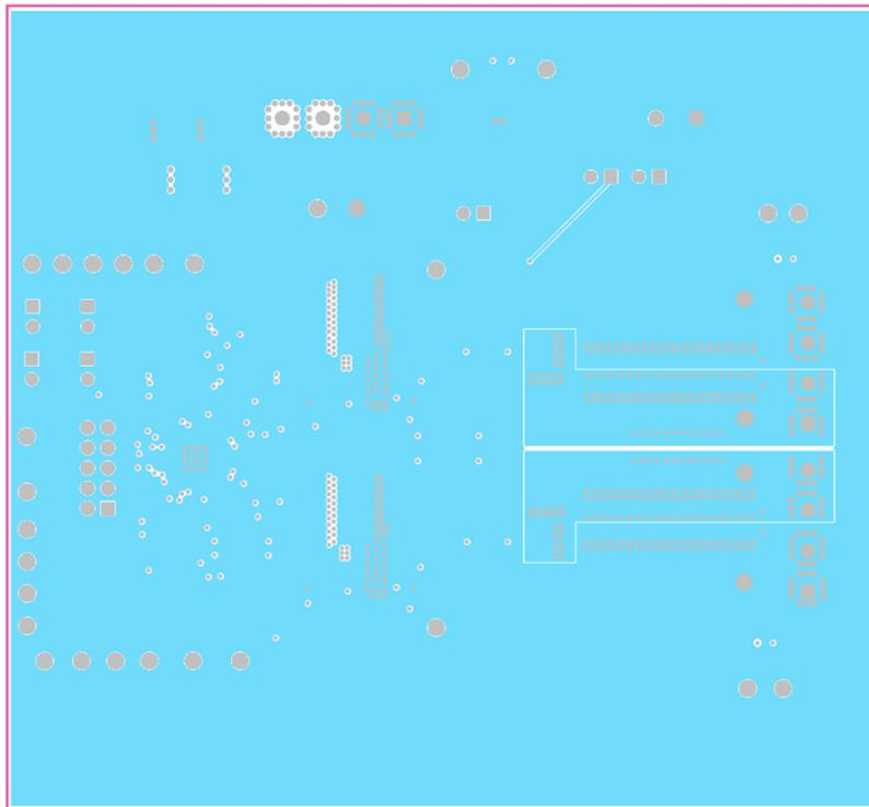
**Figure 27. PWR594 EVM Internal Layer 2 (Top View)**
