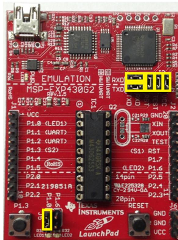
Figure 2. Proper Jumper Configuration on the LaunchPad
