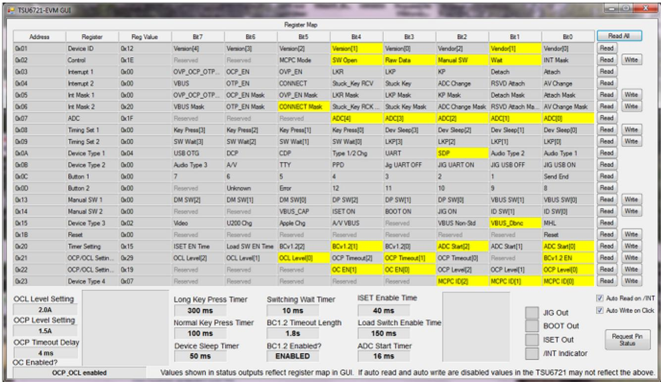
Figure 7. TSU6721EVM GUI Showing SDP Charger Detection
