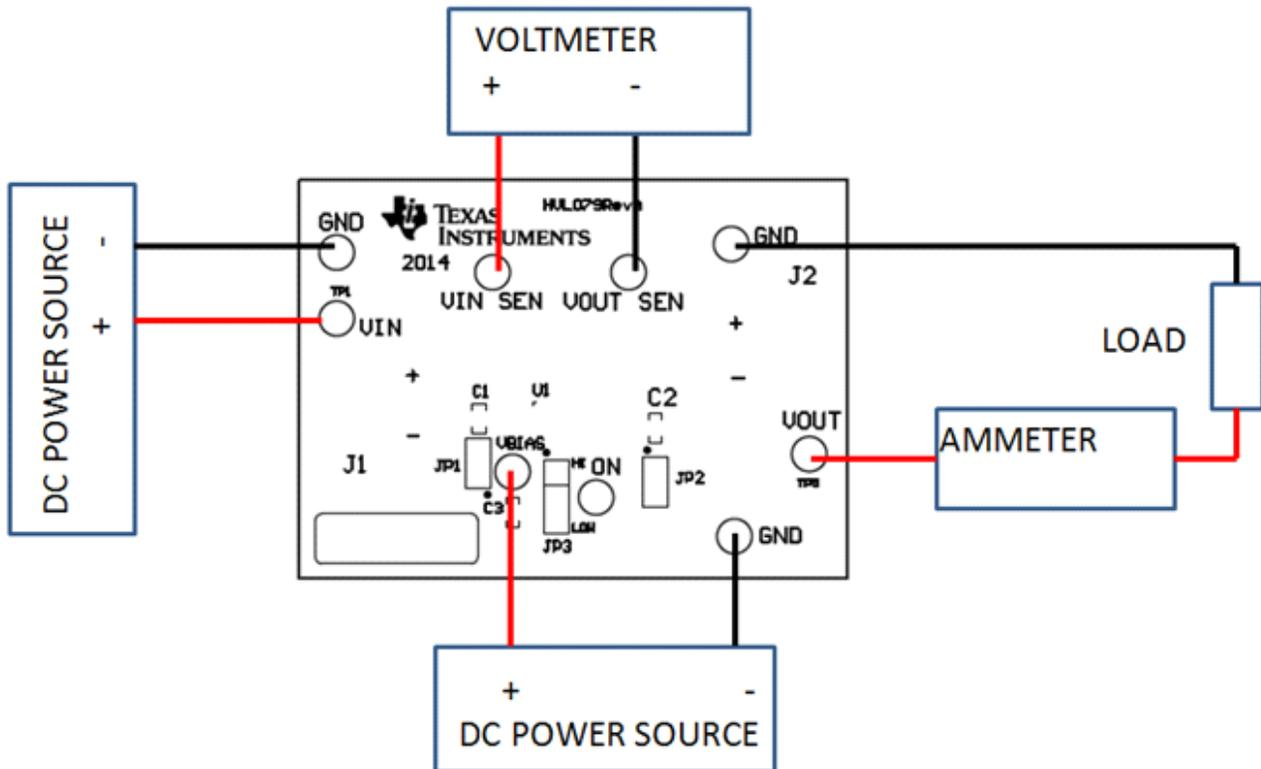
Figure 5.  $R_{ON}$  Setup
