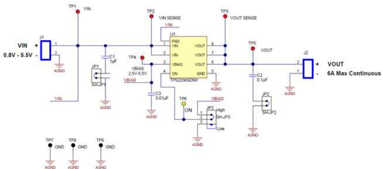
Figure 1. TPS22969EVM-079 Schematic
