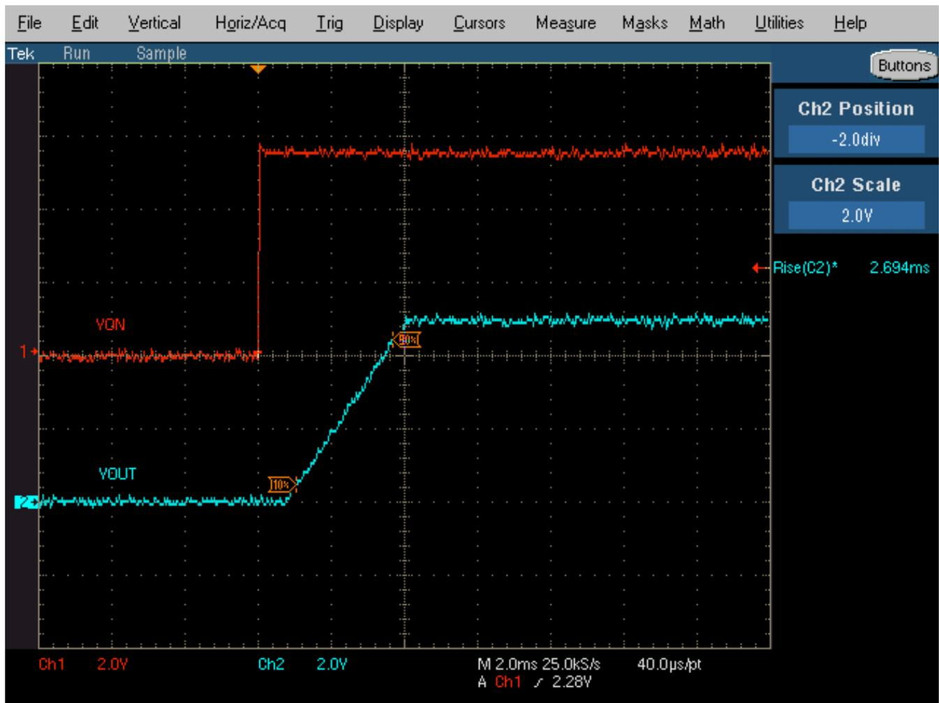
Figure 7. TPS22969 Vout  $t_R$  Example ( $V_{BIAS} = 5V$ ,  $V_{IN} = 5V$ ,  $R_L = 10\Omega$ )
