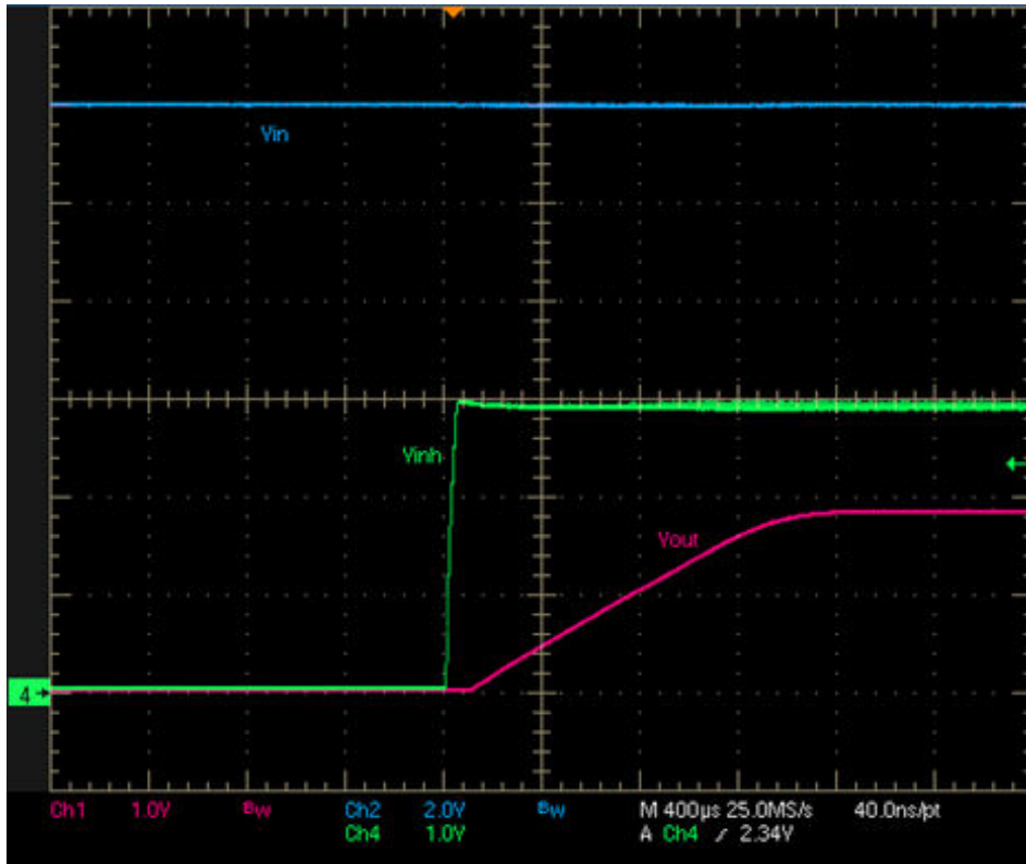
Figure 6-3. INH Start-Up Waveform
