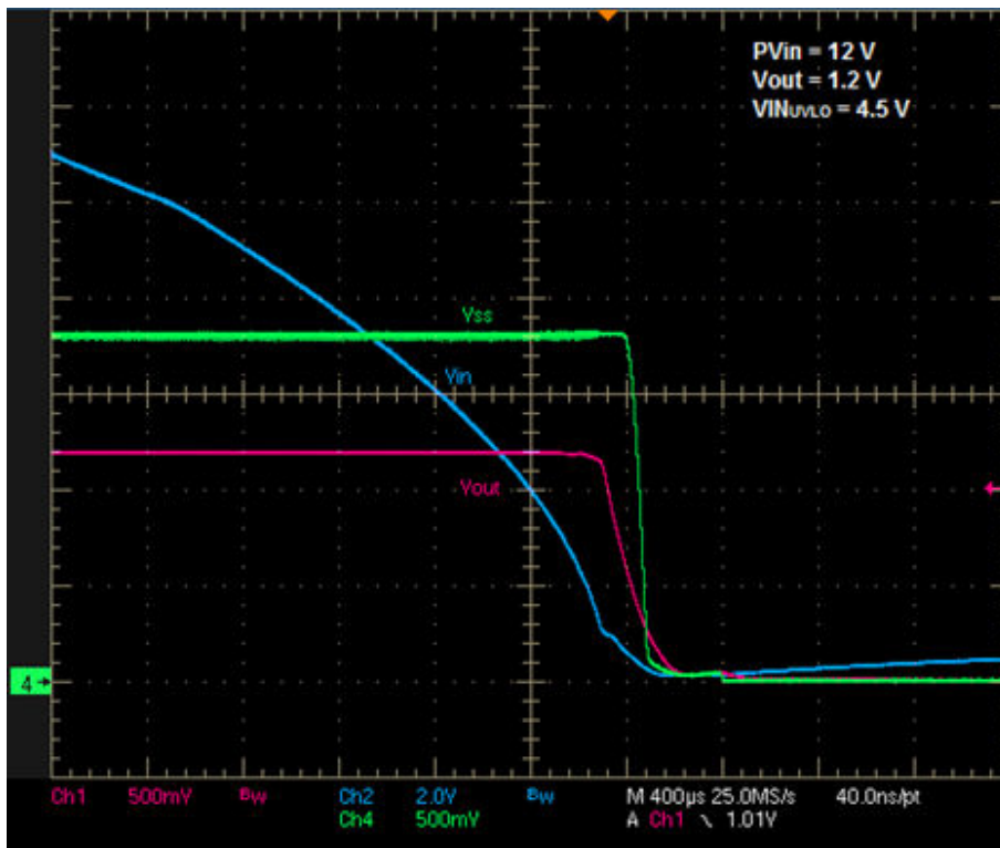
Figure 6-2. UVLO Shutdown Waveform
