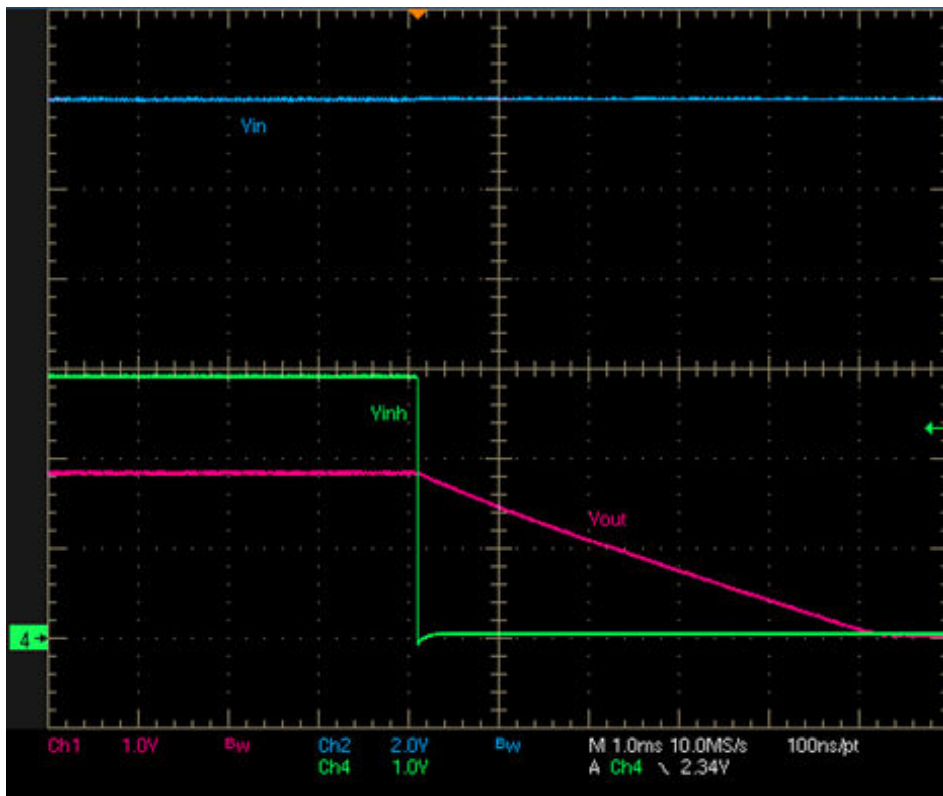
Figure 6-4. INH Shutdown Waveform
