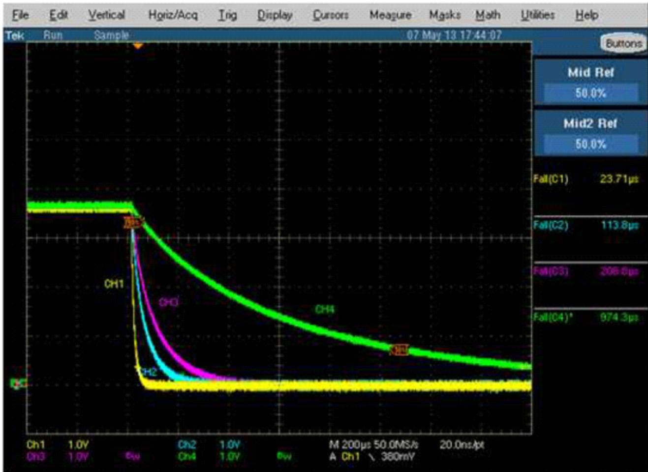
Figure 34. Programmable Output Discharge (Fall Time Control)
