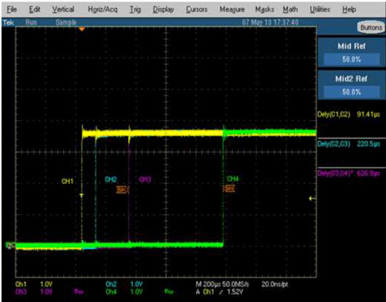
Figure 33. Programmable Turn on Delay Time
