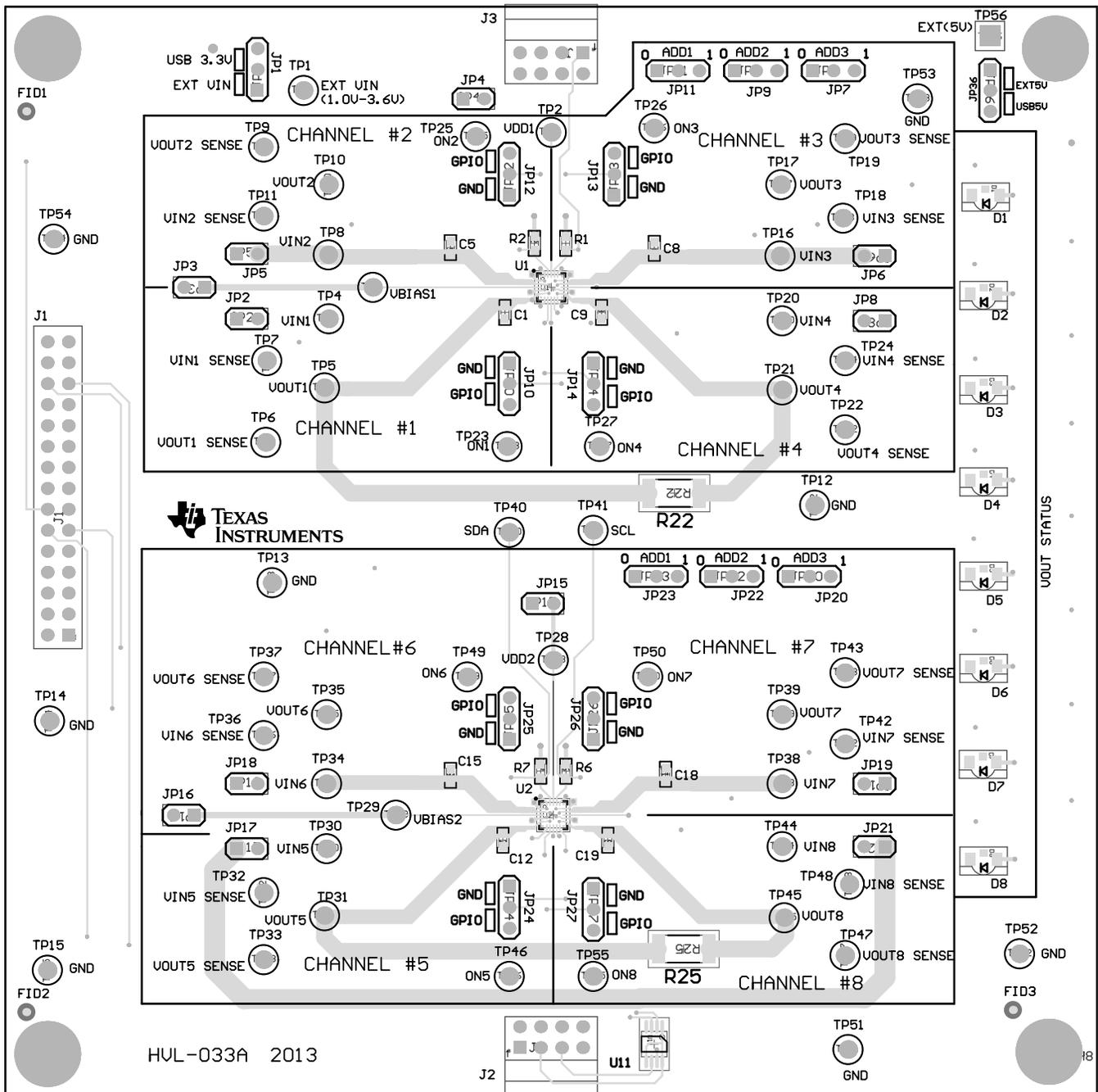
Figure 30. I<sup>2</sup>C Load Switch EVM Board Top Side (Minus GND Pour)
