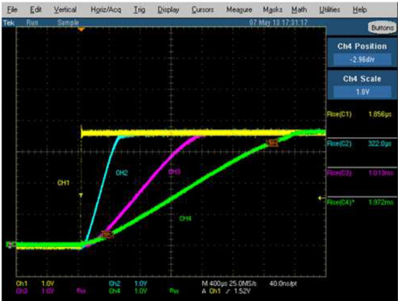
Figure 32. Programmable Slew Rate Control
