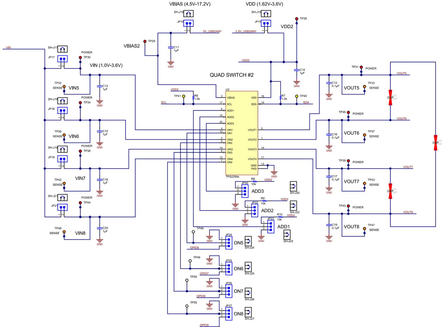
Figure 25. I<sup>2</sup>C Load Switch EVM Board Schematic (1 of 3)
