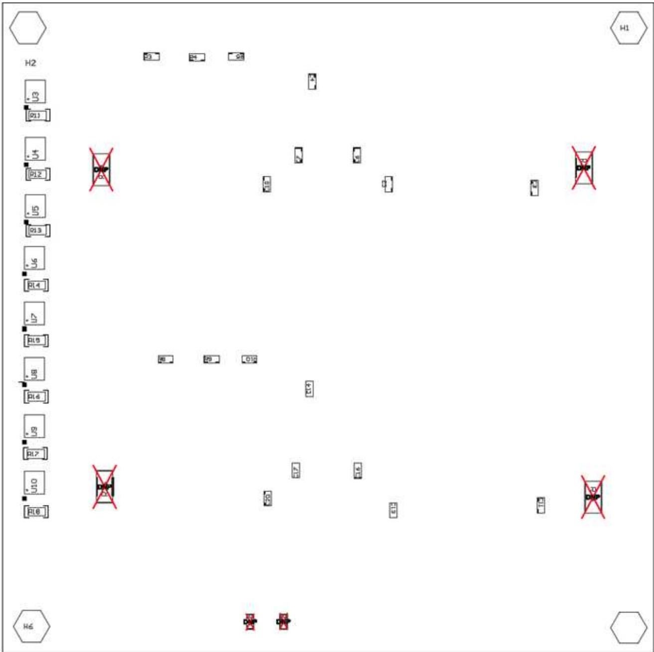
**Figure 29. I<sup>2</sup>C Load Switch EVM Board Bottom Assembly**
