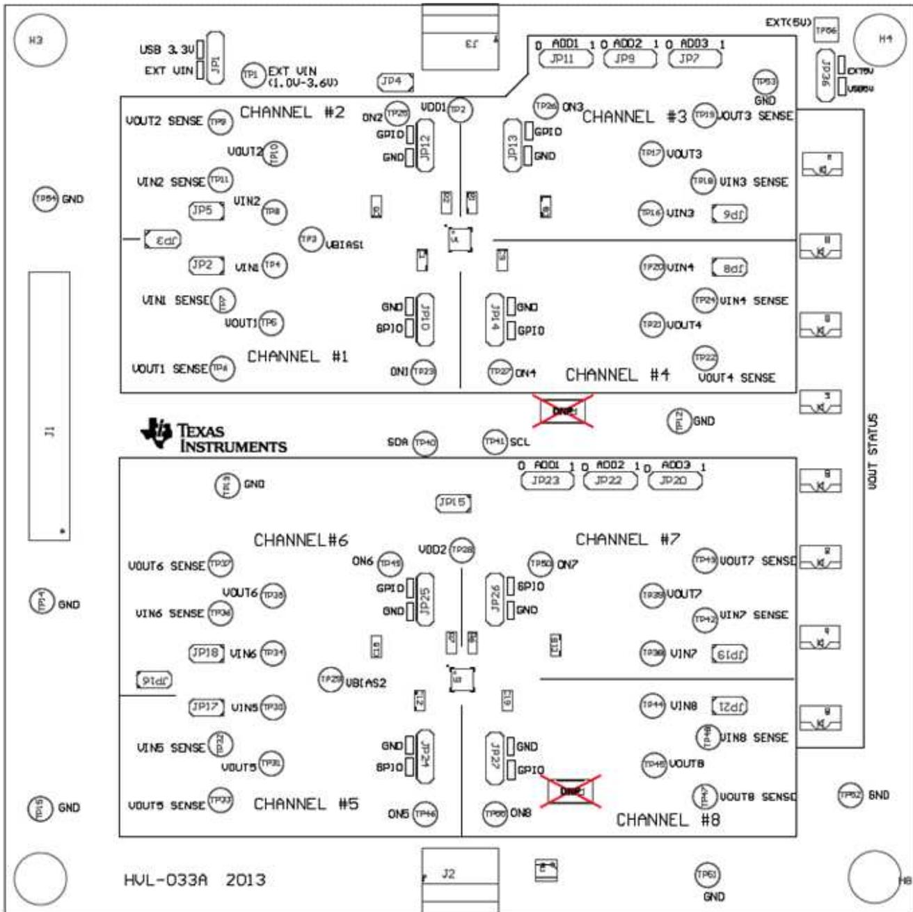
Figure 28. I²C Load Switch EVM Board Top Assembly
