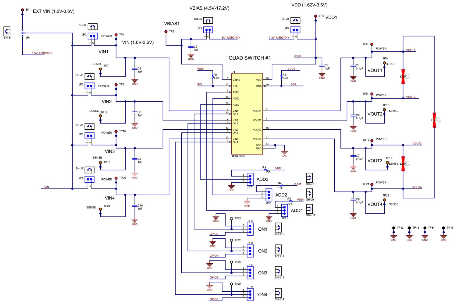
Figure 26. I<sup>2</sup>C Load Switch EVM Board Schematic (2 of 3)
