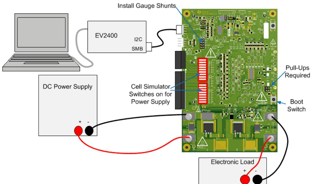
Figure 2. EVM Connection for Basic Gauge Operation
