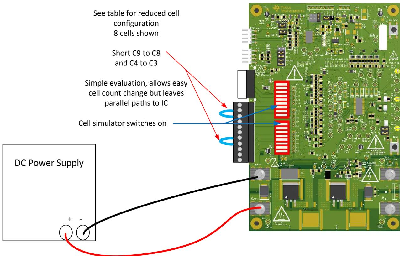
**Figure 18. Example 8 Cell Simple Evaluation Configuration**
