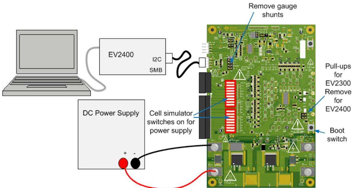
Figure 1. EVM Connection for Basic AFE Operation
