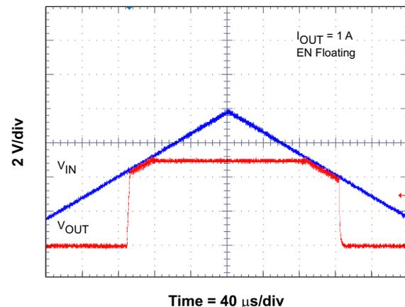
Figure 21. Low Dropout Start Up and Shutdown
