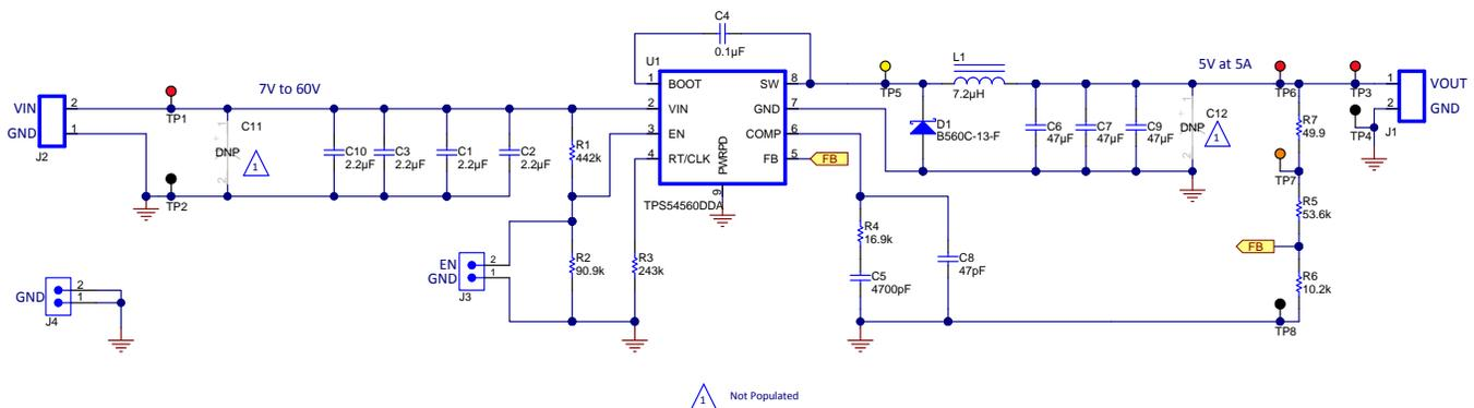
**Figure 2. TPS54560EVM-515 Schematic**
