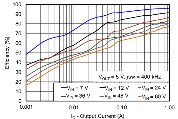
**Figure 4. Light-Load Efficiency**
