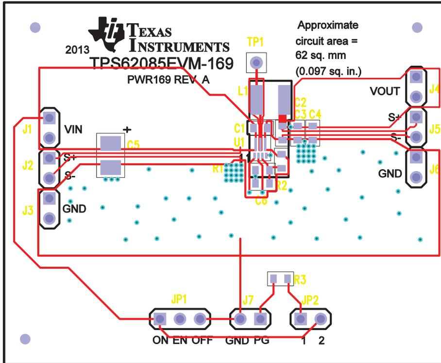
Figure 4. Assembly Layer
