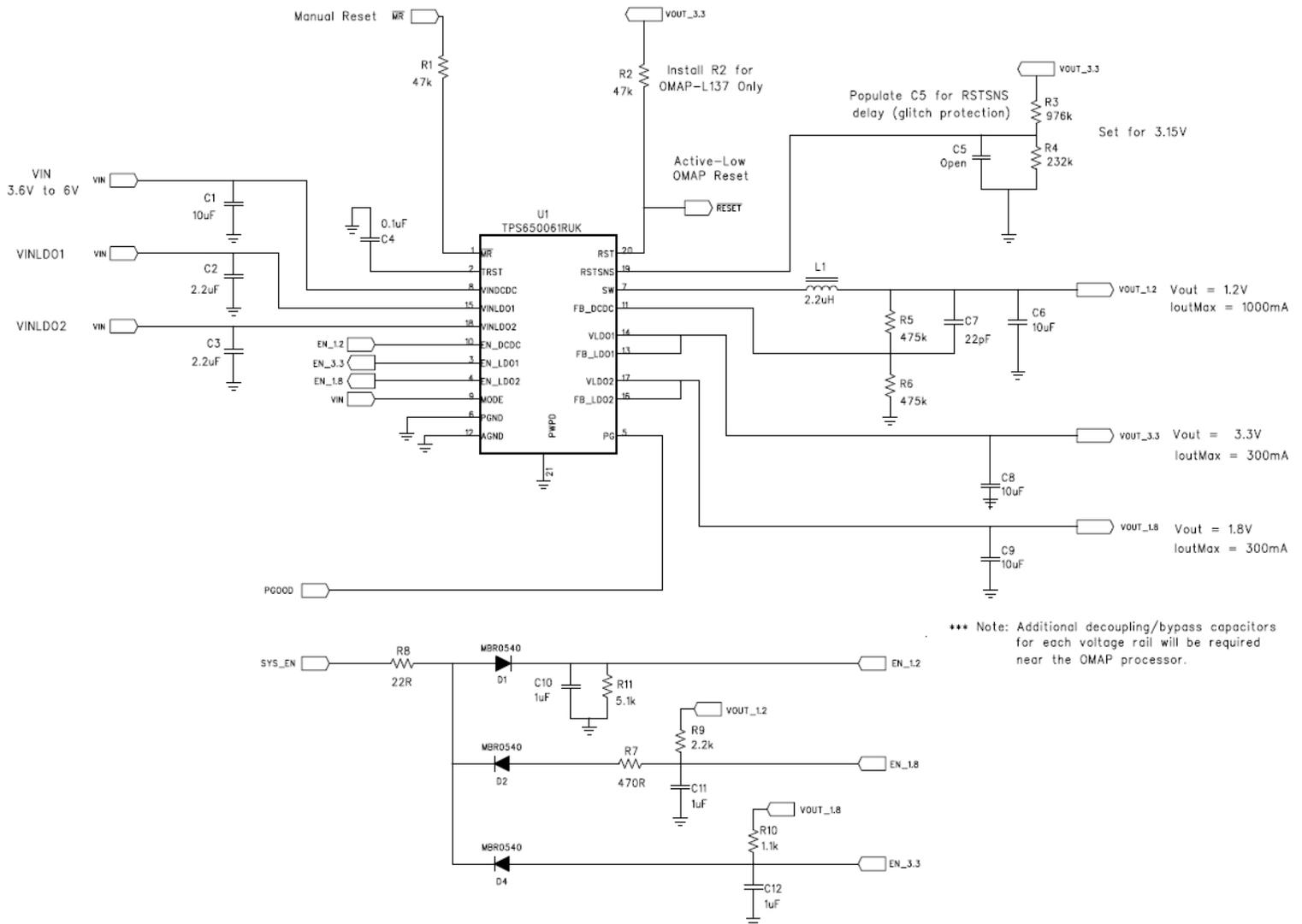
Figure 1: TPS650061 Schematic with Discrete Sequencing Components
