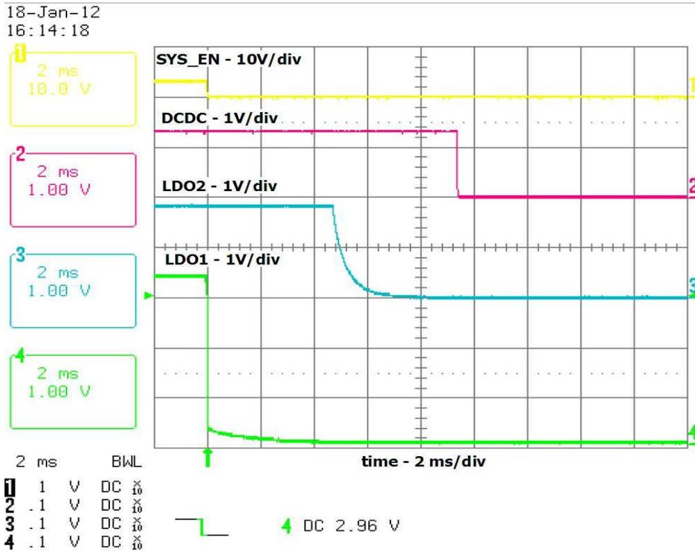
Figure 5. Power-Down Sequence With System Enable LOW
