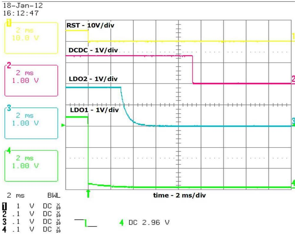
Figure 6. Power-Down Sequence and Reset Pulled LOW
