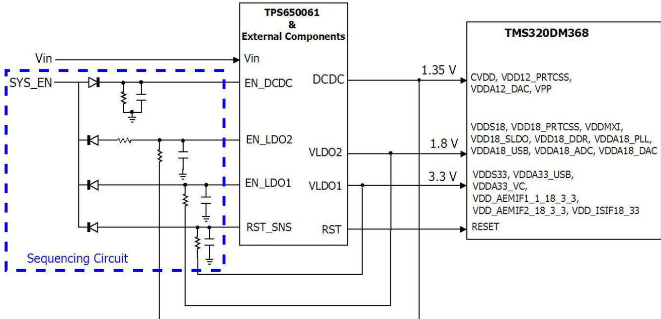
Figure 1. TPS650061 and TMS320DM368 Block Diagram
