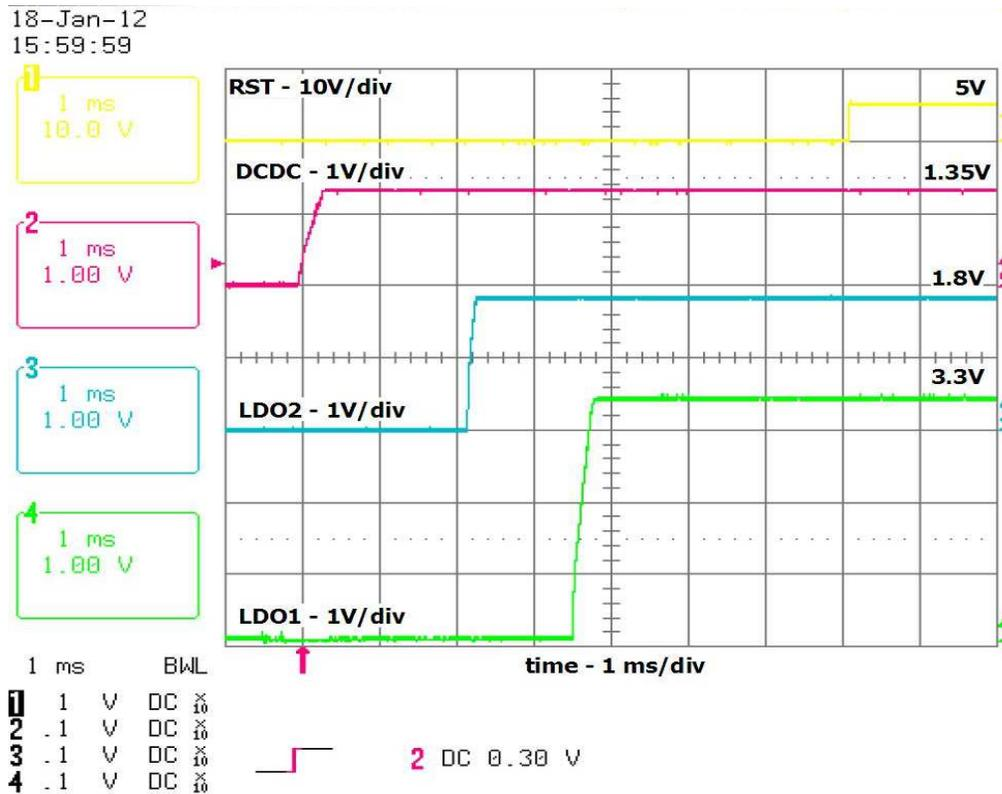
Figure 4. Power-Up Sequence and Reset Release
