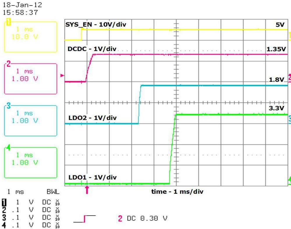
**Figure 3. Power-Up Sequence With System Enable HIGH**
