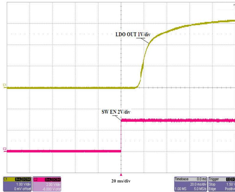
Figure 4-5. LDO Output Voltage Turn-On, SW Enable
