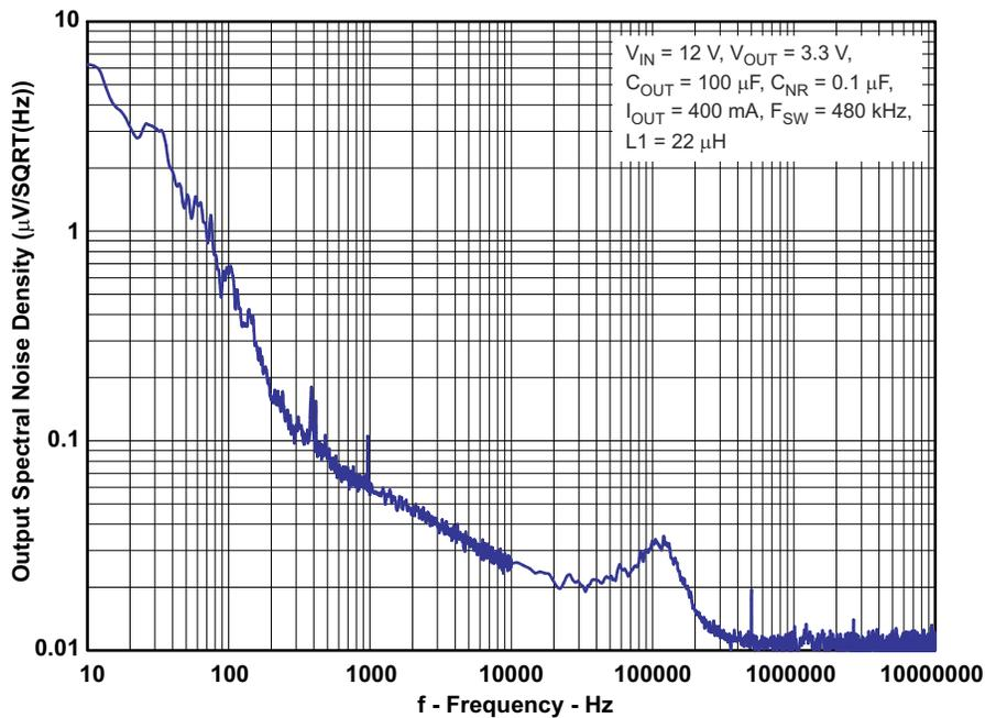
Figure 4-2. Output Spectrum Noise Density vs Frequency
