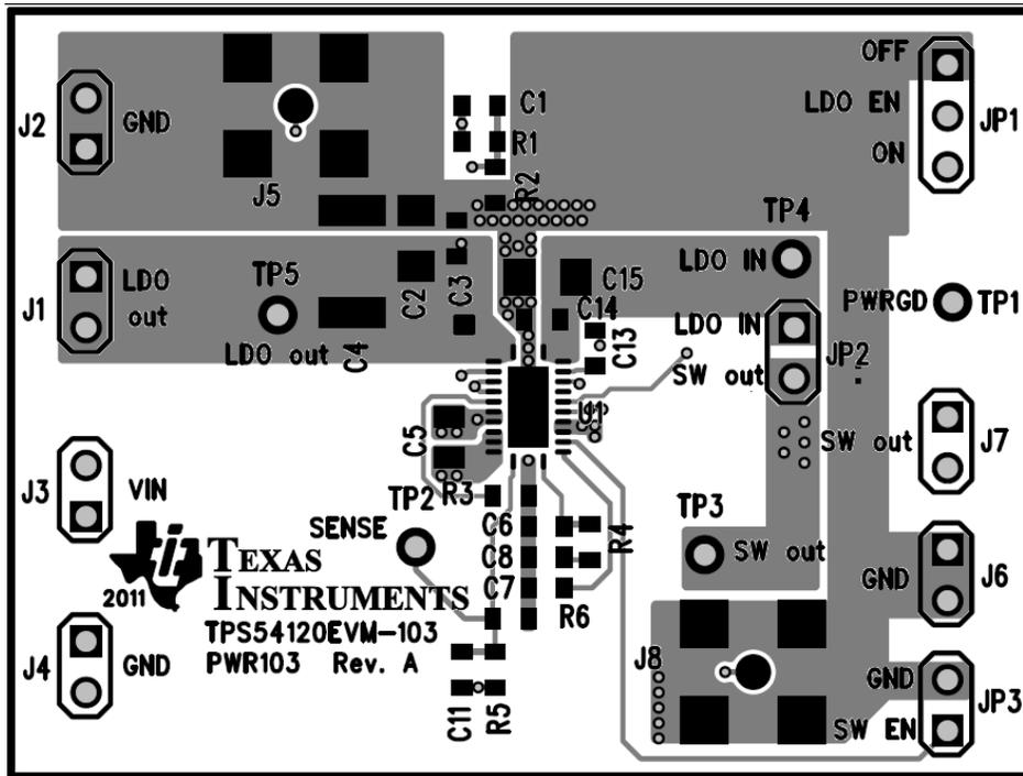
Figure 5-1. Top Side Silkscreen and Routing
