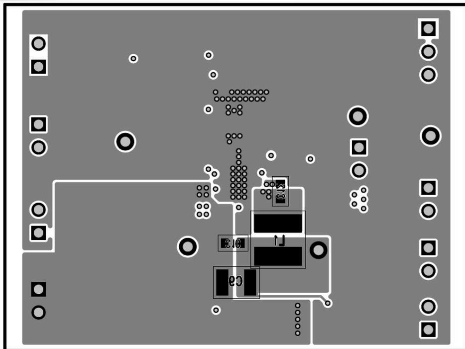
Figure 5-4. Bottom Layer Silkscreen and Routing
