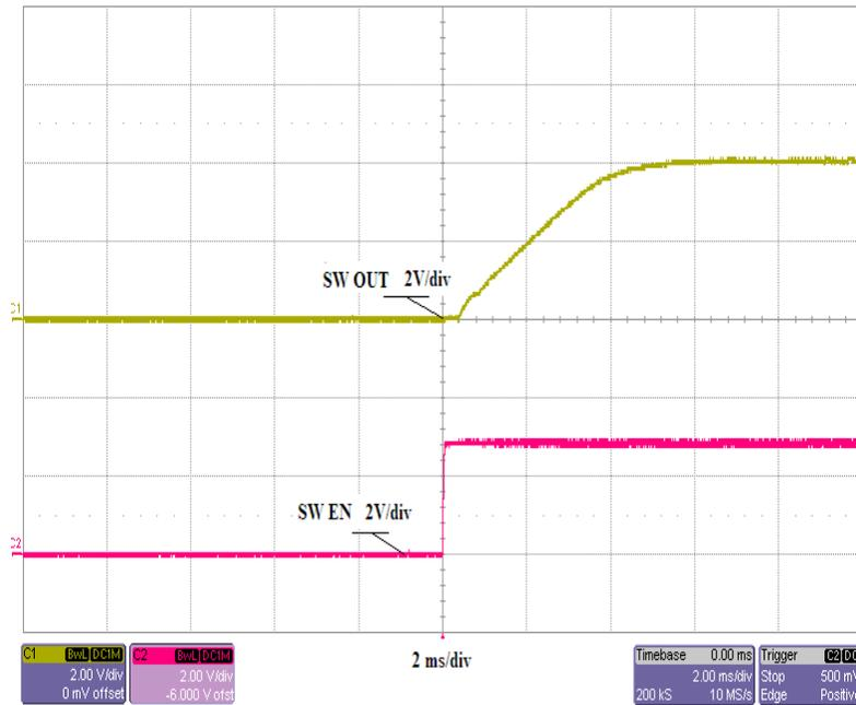
Figure 4-3. Switcher Converter Output Voltage Turn-On, SW Enable
