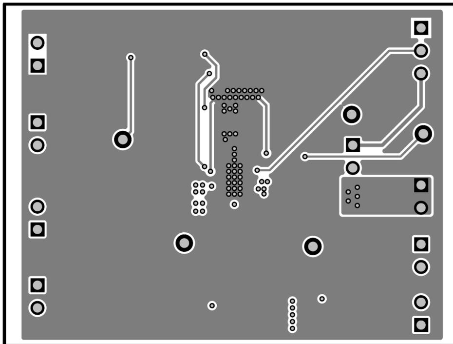
Figure 5-2. Second Layer (Internal) Routing
