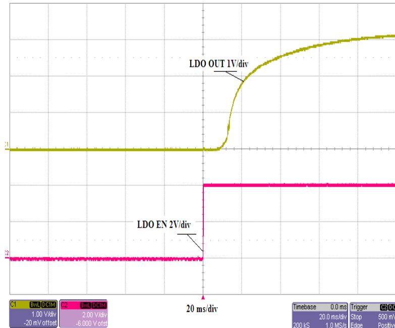
Figure 4-4. LDO Output Voltage Turn-On, LDO Enable
