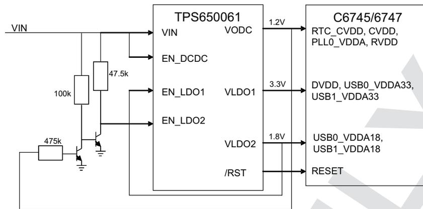
Figure 1. TPS650061 and C6745/47 Simplified Block Diagram
