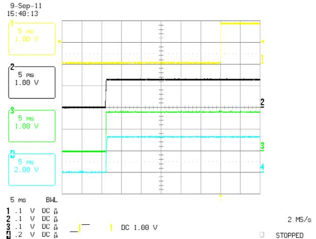
**Figure 4. TPS650061 Power-Up and RESET, Ch. 1 - RESET, Ch. 2 - 1.3V Rail, Ch. 3 - 1.8V Rail, Ch. 4 - 3.3V Rail**
