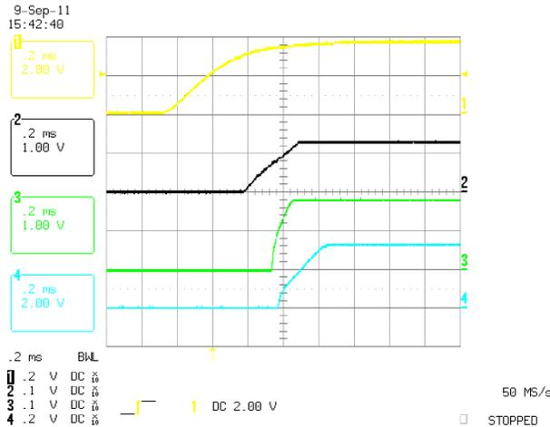
**Figure 3. TPS650061 Power-Up, Ch. 1 - VIN, Ch. 2 - 1.3V Rail, Ch. 3 - 1.8V Rail, Ch. 4 - 3.3V Rail**
