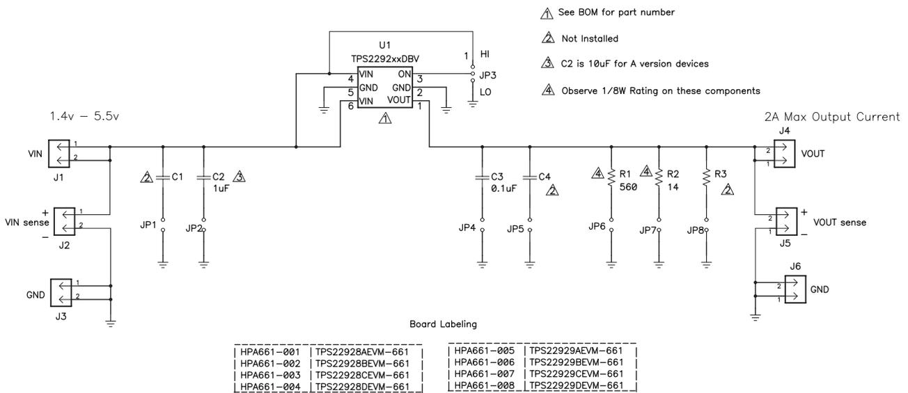
Figure 4. TPS2292xxEVM-661 Schematic
