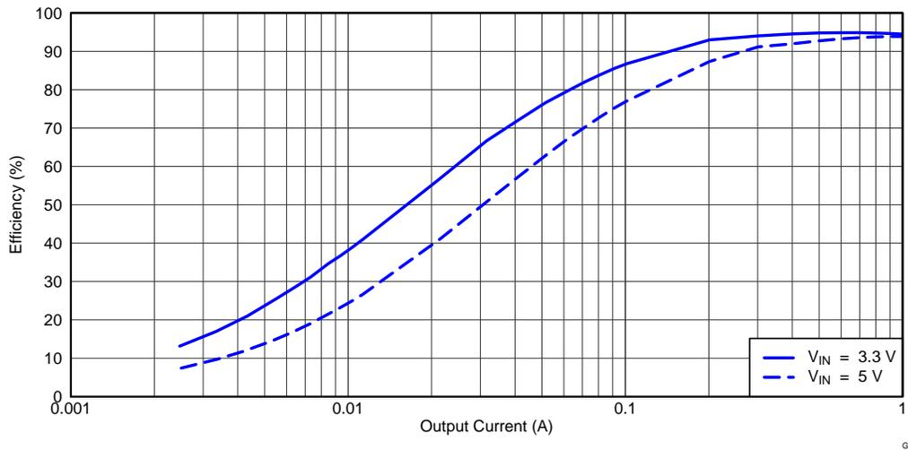
**Figure 2. TPS54519EVM-037 Low Current Efficiency**
