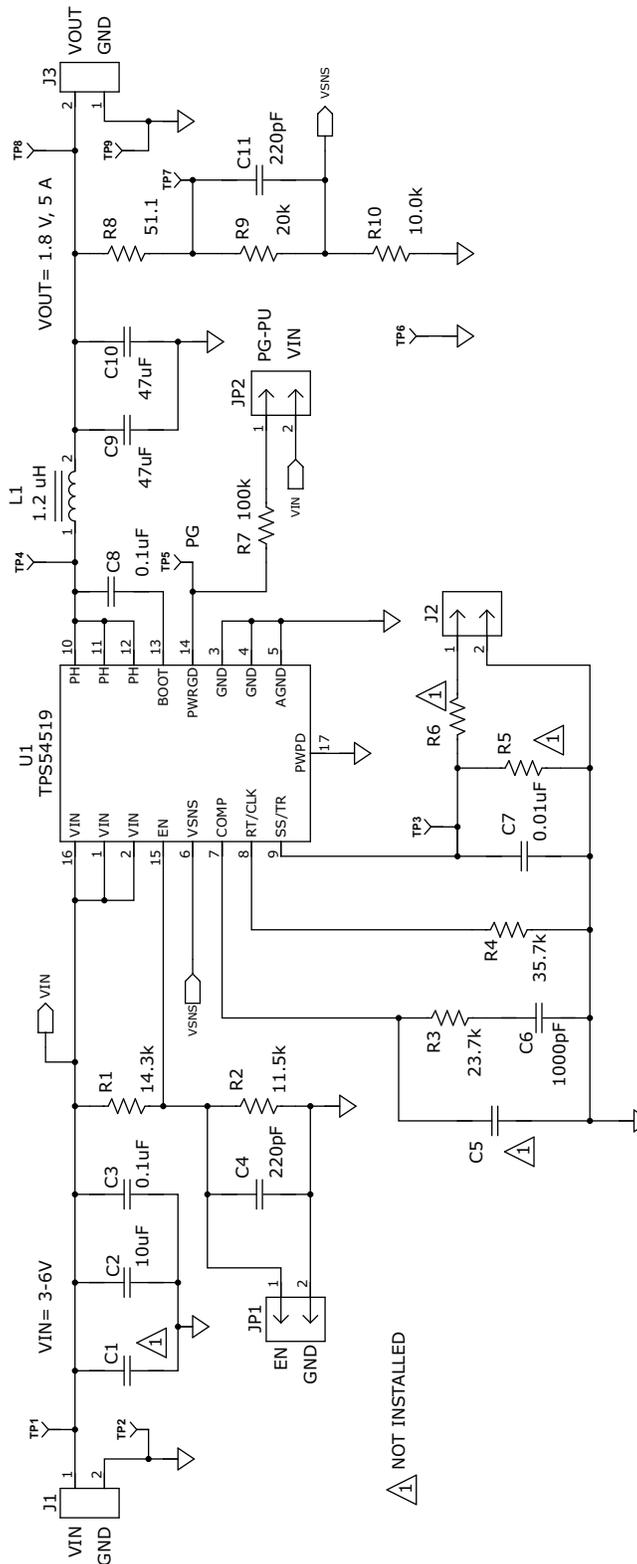
Figure 18. TPS54519EVM-037 Schematic
