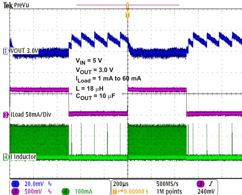
Figure 7. TPS62122 Load Transient Response
