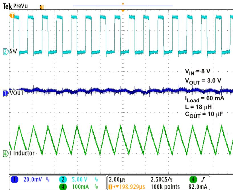
Figure 8. TPS62122EVM Output Ripple, 60-mA Load
