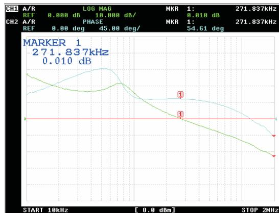
Conditions: VIN = 5.0 V, VOUT = 1.8 V, I<sub>OUT</sub> = 1.6 A; bandwidth: 271 kHz, phase margin: 54°
