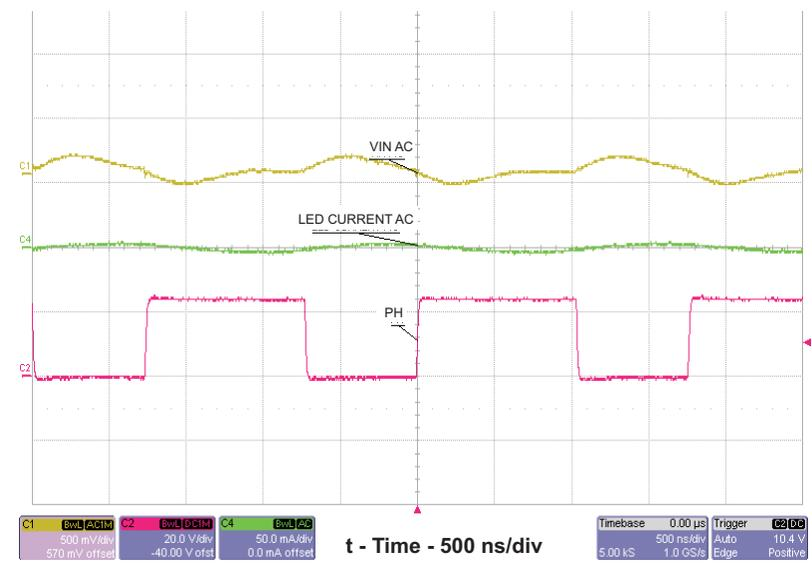
Figure 7. Input Voltage Ripple, Vin=24.0V, Iout=675mA, AC Coupled
