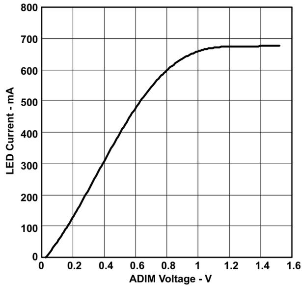
Figure 10. Analog Dimming, LED Current vs. ADIM Voltage
