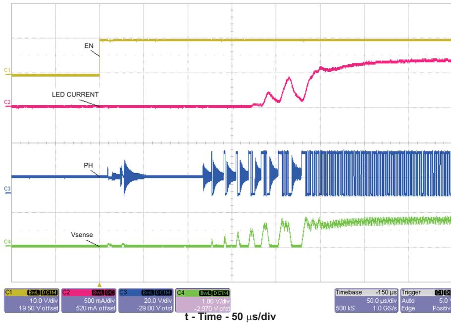
Figure 8. Start-up relative to EN, Vin=24V, Iout=675mA
