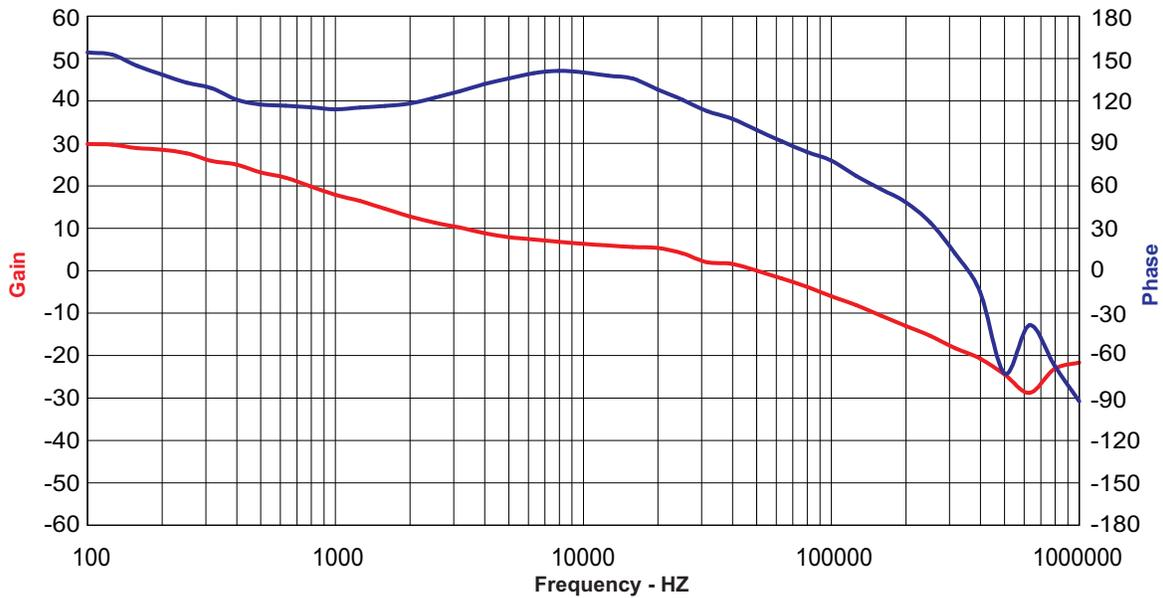
Figure 11. Loop response, VIN = 24V, Iout = 675mA
