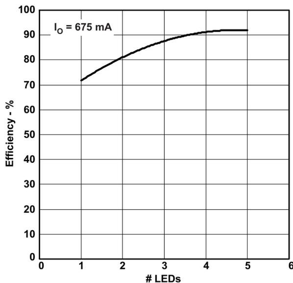
Figure 5. Efficiency, Vin=24V
