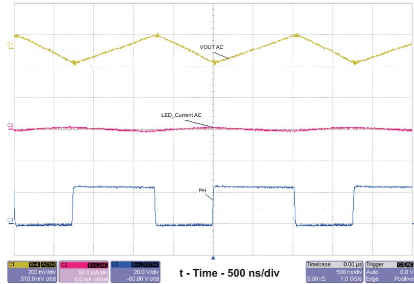
Figure 6. Output Ripple, Vin=24.0V, Iout=675mA, AC Coupled
