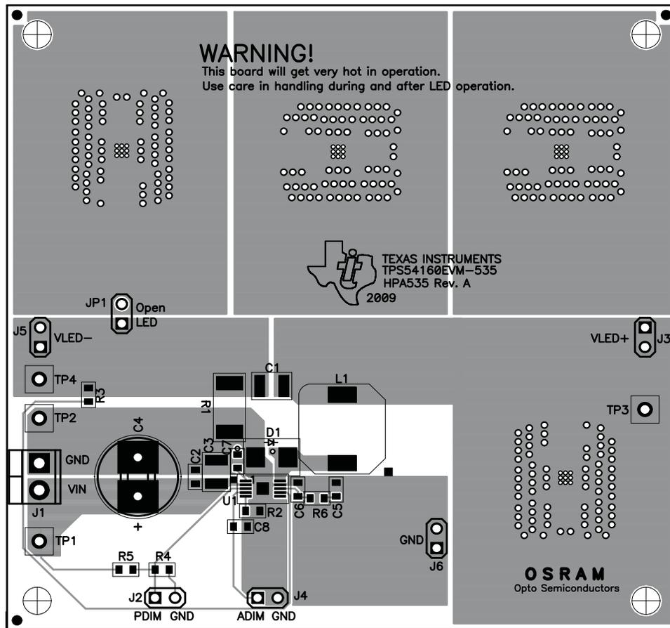
Figure 2. Top Assembly Layer
