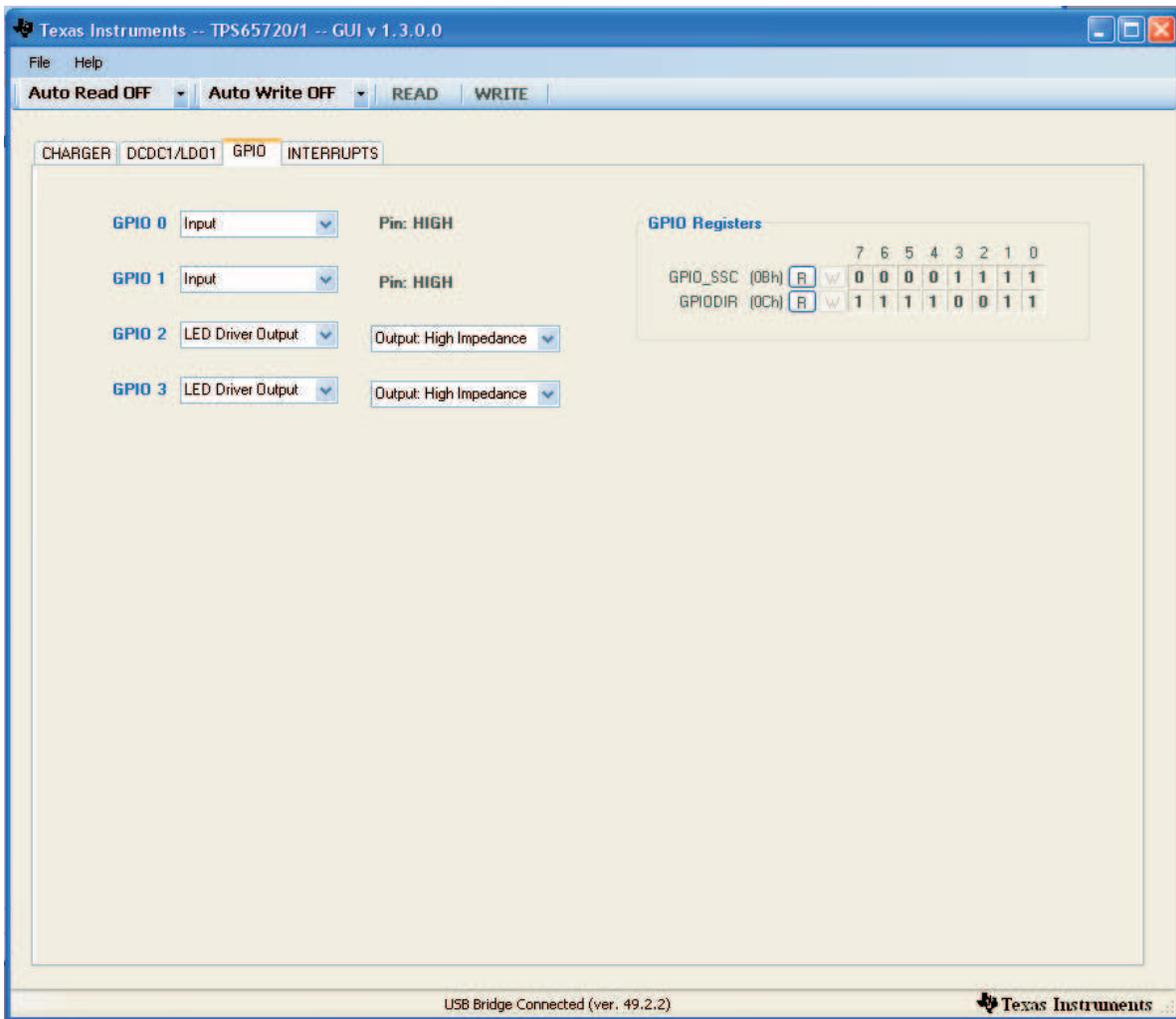
Figure 6. GPIO View
