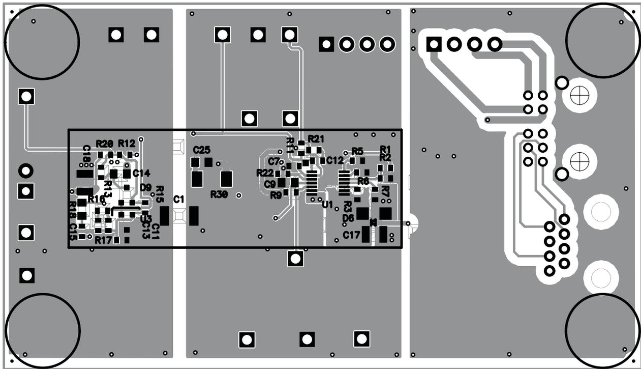
**Figure 9. Bottom-Side Placement**
