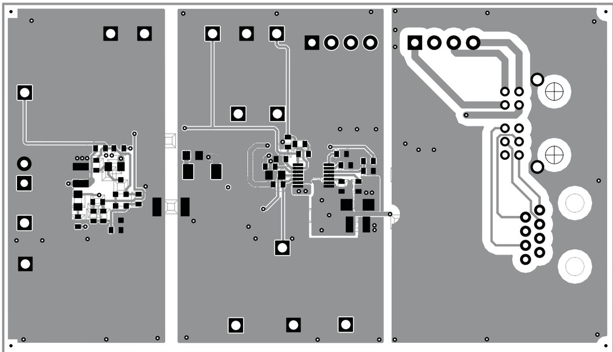
**Figure 8. Bottom-Side Routing**
