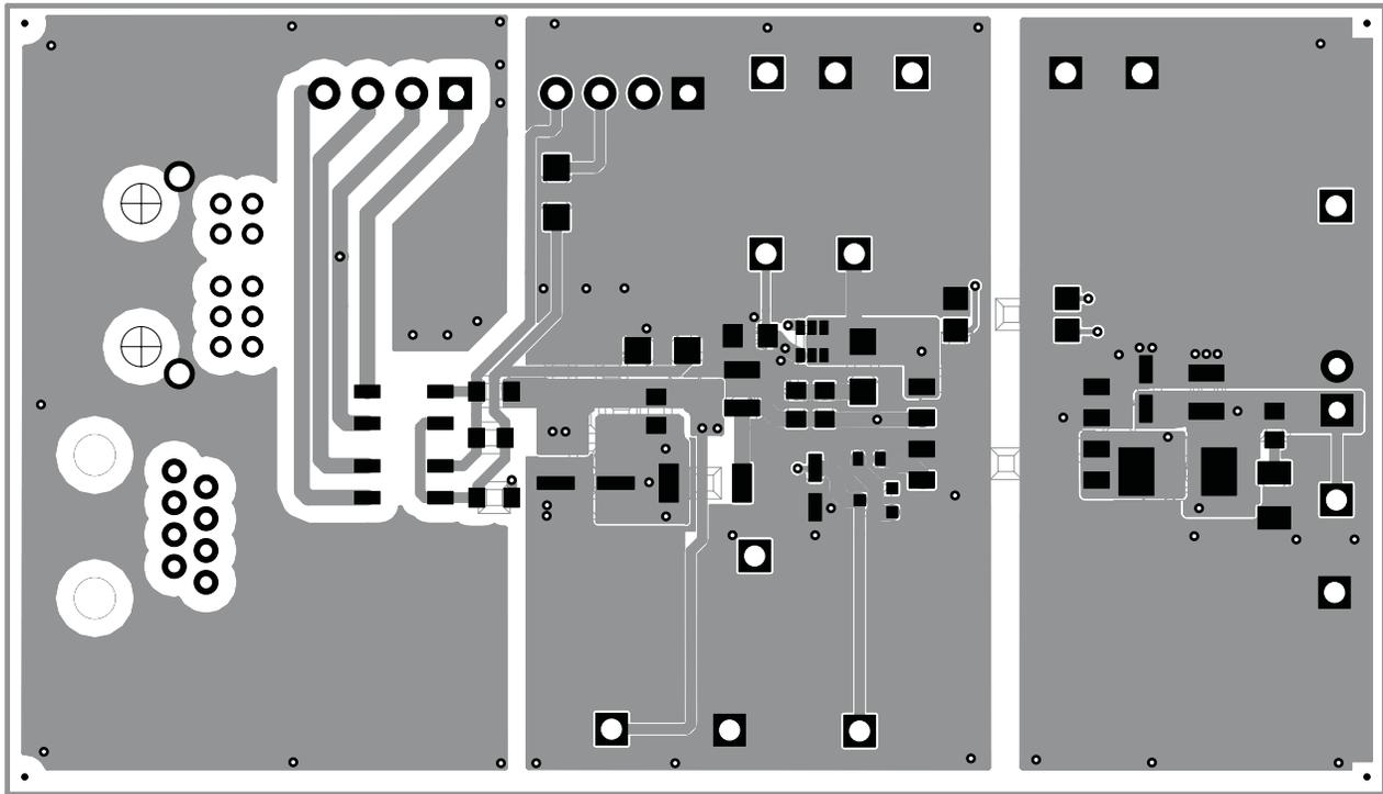
**Figure 7. Top-Side Routing**
