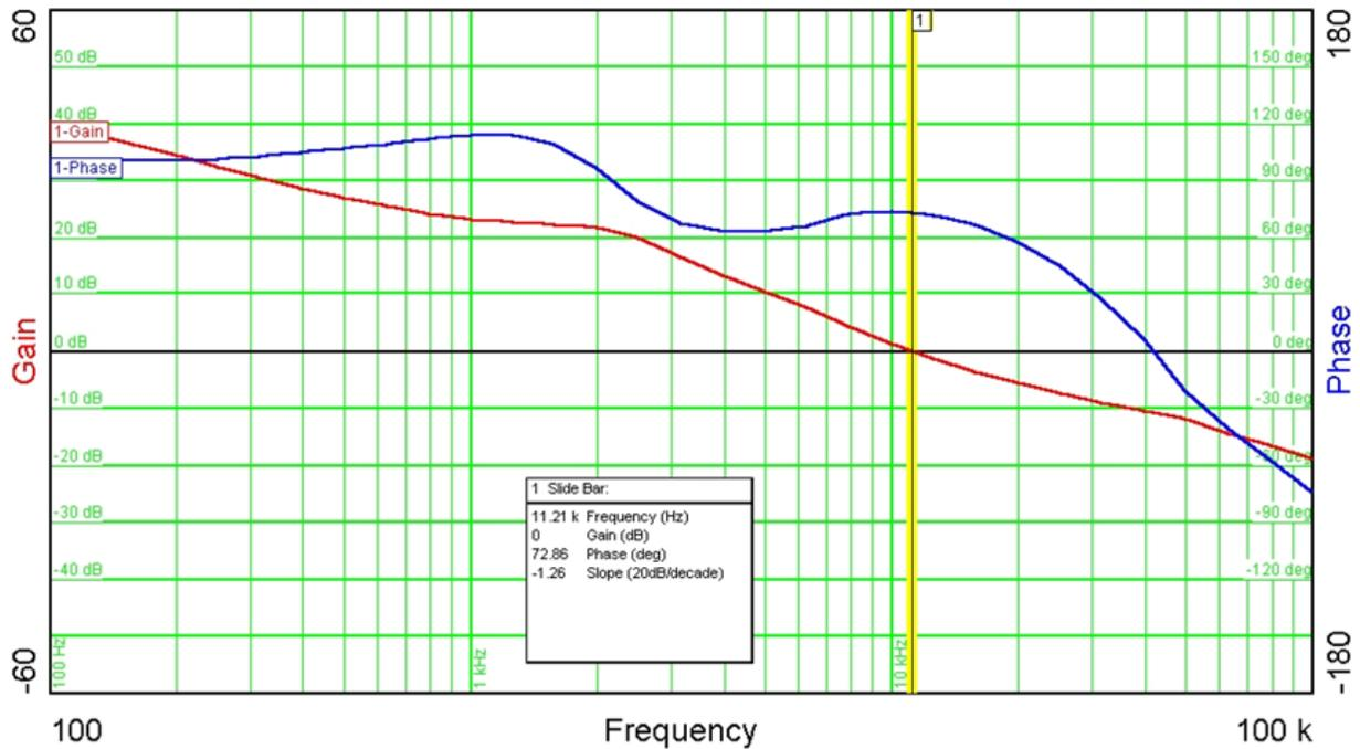
Figure 4. Measured Loop Response, TPS5430,  $V_{IN} = 12$  V
