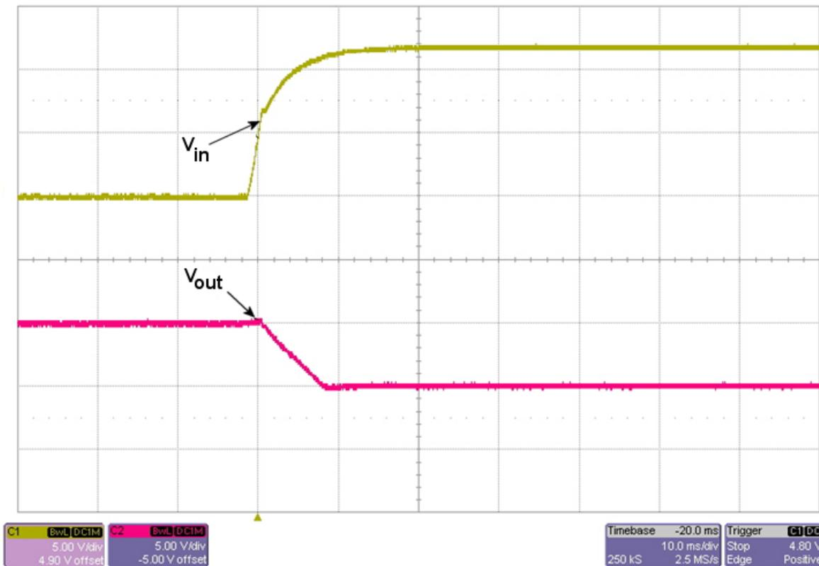
Figure 6. Power Up,  $V_{OUT}$  Relative to  $V_{IN}$
