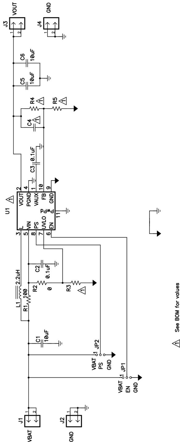
Figure 6. TPS6120xEVM-179 Schematic
