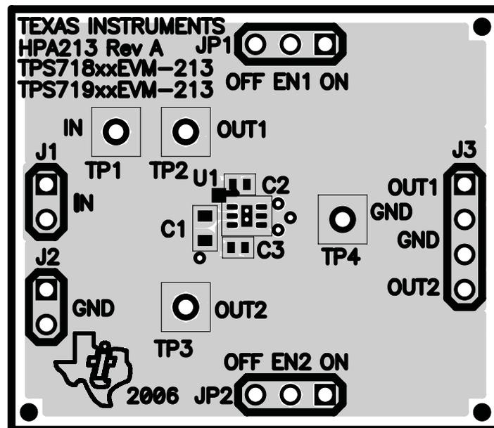
Figure 1. Assembly Layer
