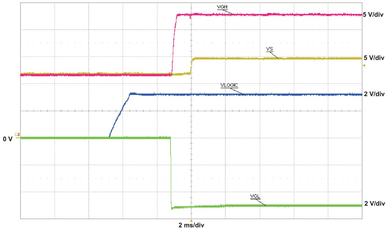
Figure 3. Power-Up Sequencing With EN2 = VIN
