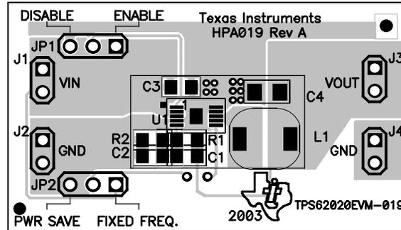
Figure 3-3 shows the PCB layout top layer
