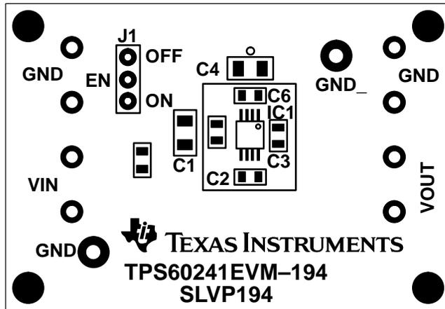
The total space required for the IC and the capacitors on the EVM is only about  $10\text{ mm} \times 12\text{ mm} = 120\text{ mm}^2$ . The capacitors are not optimized for space. They are optimized for performance. It is possible to use smaller capacitors to optimize the layout for minimum board space. On the EVM, it is also possible to solder some other capacitors because 1206-size pads have been added in parallel to  $C_{IN}$  and  $C_{OUT}$ .
