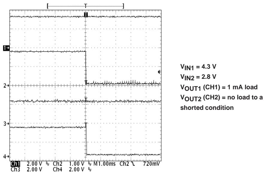
In Figure 4–9,  $V_{OUT2}$  is pulsed into a shorted condition. Because SEQUENCE is high,  $V_{OUT1}$  is disabled after the internal current limit circuitry disables  $V_{OUT2}$ . PG1 (CH3), which is tied to  $\overline{MR1}$ , goes low when  $V_{OUT1}$  falls below 95% of its regulated voltage.  $\overline{RESET}$  (CH4) goes low when  $V_{OUT2}$  falls below 95% of its regulated voltage.
