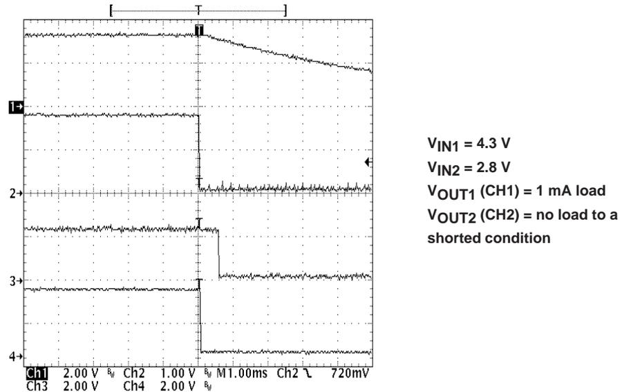
In Figure 4–10,  $\overline{MR}$  (CH3) is toggled low and  $\overline{RESET}$  (CH4) follows  $\overline{MR1}$ .  $V_{OUT1}$  (CH1) and  $V_{OUT2}$  (CH2) are unaffected.
