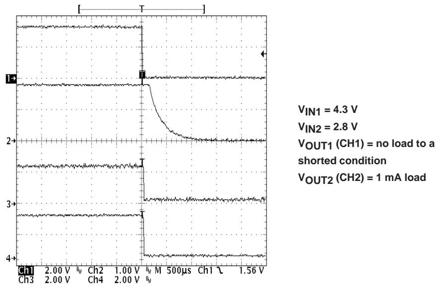
In Figure 4–7,  $V_{OUT1}$  (CH1) is pulsed into a shorted condition. Because SEQUENCE is high,  $V_{OUT2}$  (CH2) is not disabled after the internal current limit circuitry disables  $V_{OUT1}$ . PG1 (CH3), which is tied to  $\overline{MR1}$ , goes low when  $V_{OUT1}$  falls below 95% of its regulated voltage.  $\overline{RESET}$  (CH4) follows  $\overline{MR1}$ .
