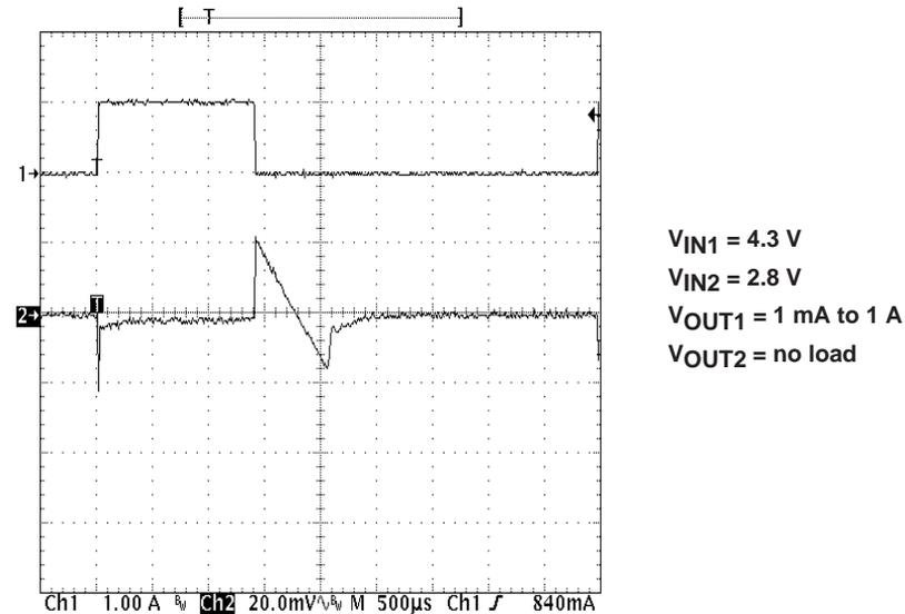
In Figure 4–2, the onboard transient generator is used to pulse  $I_{OUT2}$  (CH1) on  $V_{OUT2}$  (CH2–AC) from 1 mA to 2 A. A current loop was added to the board to measure the load current.
