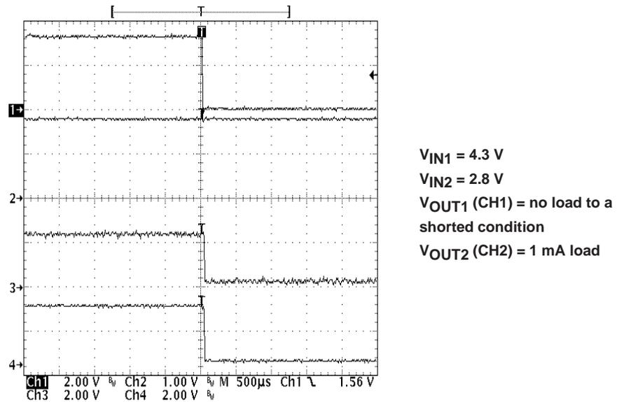
In Figure 4–8,  $V_{OUT2}$  (CH2) is pulsed into a shorted condition. Because SEQUENCE is low,  $V_{OUT1}$  (CH1) is not disabled after the internal current limit circuitry disables  $V_{OUT2}$ . PG1 (CH3), which is tied to  $\overline{MR1}$ , stays high.  $\overline{RESET}$  (CH4) goes low when  $V_{OUT2}$  falls below 95% of its regulated voltage.
