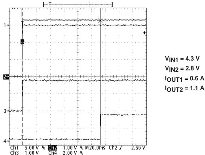
In Figure 4–6,  $V_{\text{OUT1}}$  (CH1) is pulsed into a shorted condition. Because  $\text{SEQUENCE}$  is low,  $V_{\text{OUT2}}$  (CH2) is disabled after the internal current limit circuitry disables  $V_{\text{OUT1}}$ . PG1 (CH3), which is tied to  $\overline{\text{MR1}}$ , goes low when  $V_{\text{OUT1}}$  falls below 95% of its regulated voltage.  $\overline{\text{RESET}}$  (CH4) follows  $\overline{\text{MR1}}$ .
