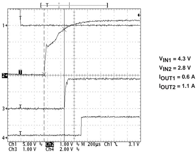
In Figure 4–5,  $\overline{\text{ENABLE}}$  (CH1) is pulsed.  $\text{SEQUENCE}$  can be either low or high. With PG1 tied to  $\overline{\text{MR1}}$ ,  $\overline{\text{RESET}}$  (CH4) goes high 120 ms after both  $V_{\text{OUT1}}$  and  $V_{\text{OUT2}}$  have reached 95% of their respective regulated output voltages.
