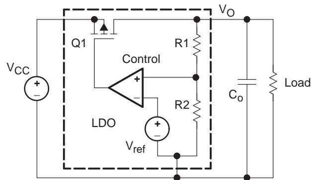
In the LDO application shown in Figure 1–1, the LDO regulates the output voltage  $V_O$ .
