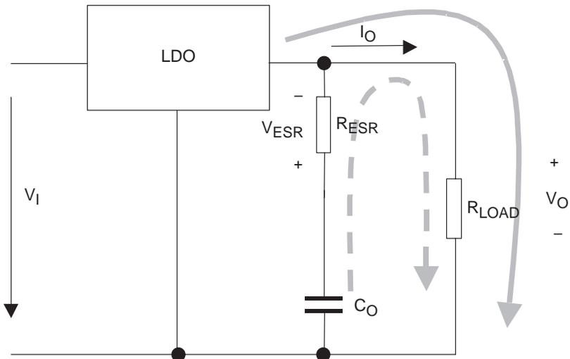
In steady state (dc state condition), the load current is supplied by the LDO (solid arrow) and the voltage across the capacitor is the same as the output voltage ( $V(C_O) = V_O$ ). This means no current is flowing into or out of the  $C_O$  branch.
