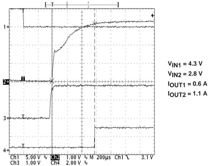
In Figure 4-3,  $\overline{\text{ENABLE}}$  (CH1) is pulsed. When SEQ is low,  $V_{\text{OUT2}}$  (CH3) powers up after  $V_{\text{OUT1}}$  (CH2) reaches 85% of its regulated output. PG1 (CH4), which is tied to  $\overline{\text{MR1}}$ , goes high when  $V_{\text{OUT1}}$  reaches 95% of its regulated voltage.
