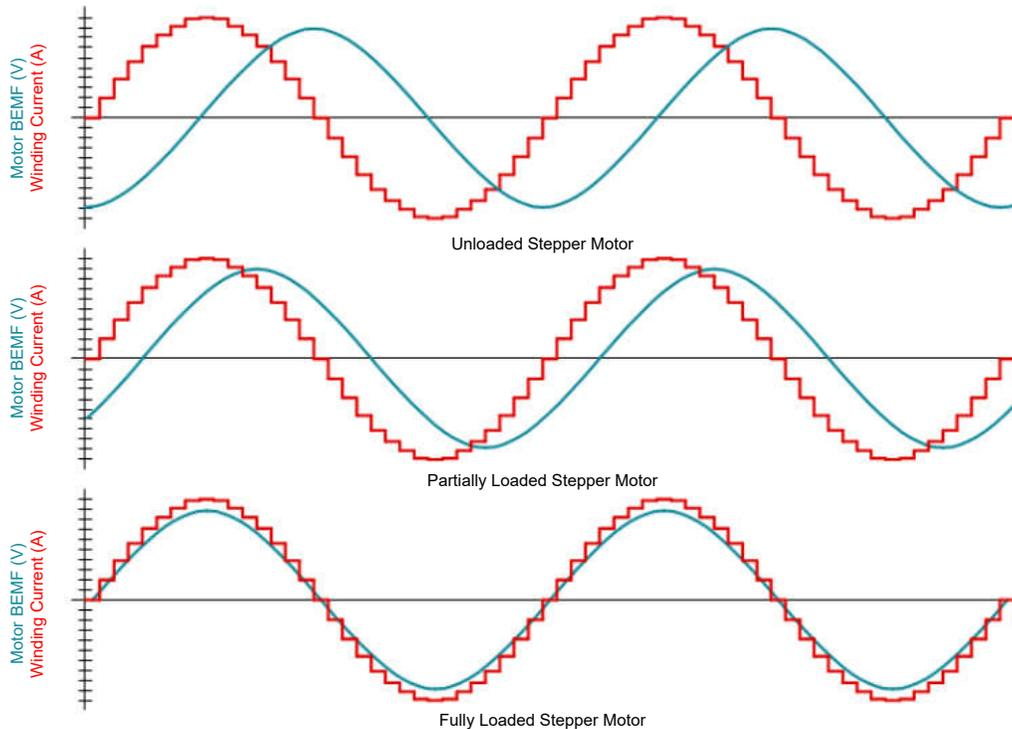
**Figure 4. Stall Detection by Monitoring Motor Back-EMF**
