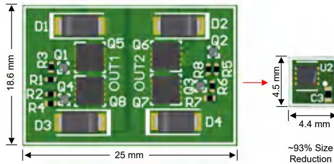
**Figure 2. Discrete vs DRV8210 and DRV8220 Layout Size**
