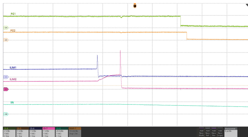
Figure 8-9. Parallel Devices Load Current During Steady State and Overload
