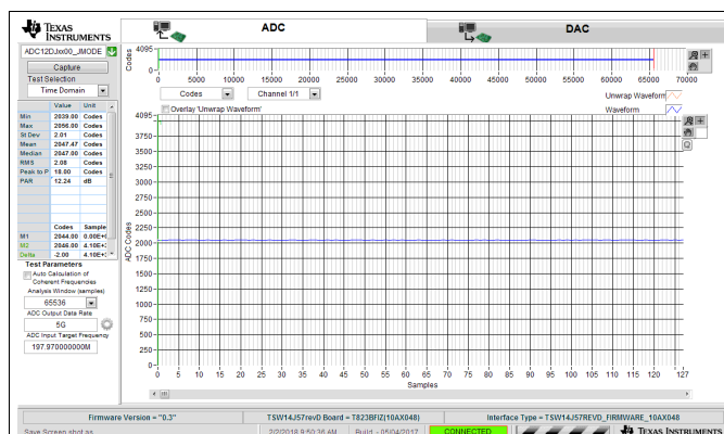
Figure 185. Idle-Channel Noise (No Input) for 5-GSPS, Single-Channel Oscilloscope
