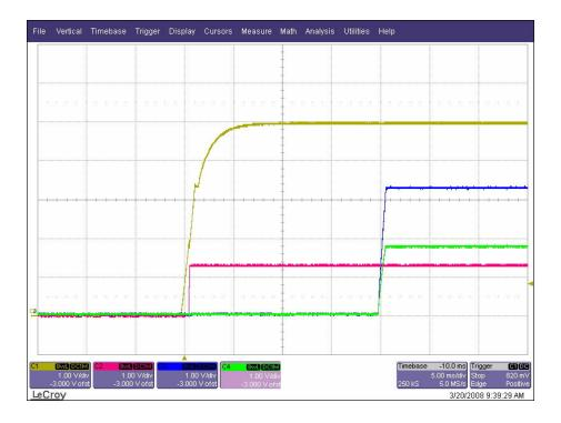
PMP3214 Power-down Sequence: TPS65053 Power for DM335 / DM355
