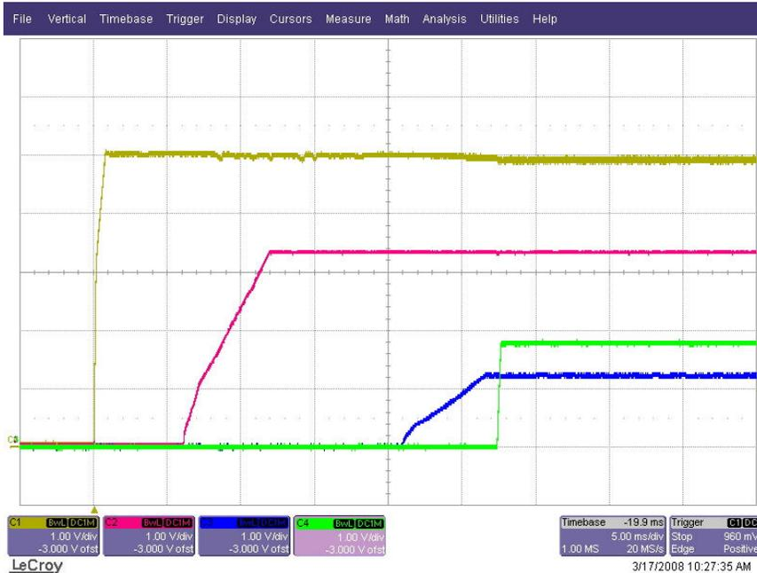
Output voltage turn-on response (traces, top to bottom, are: 1.8V, 1.5V, 1.25V, 1.2V):
