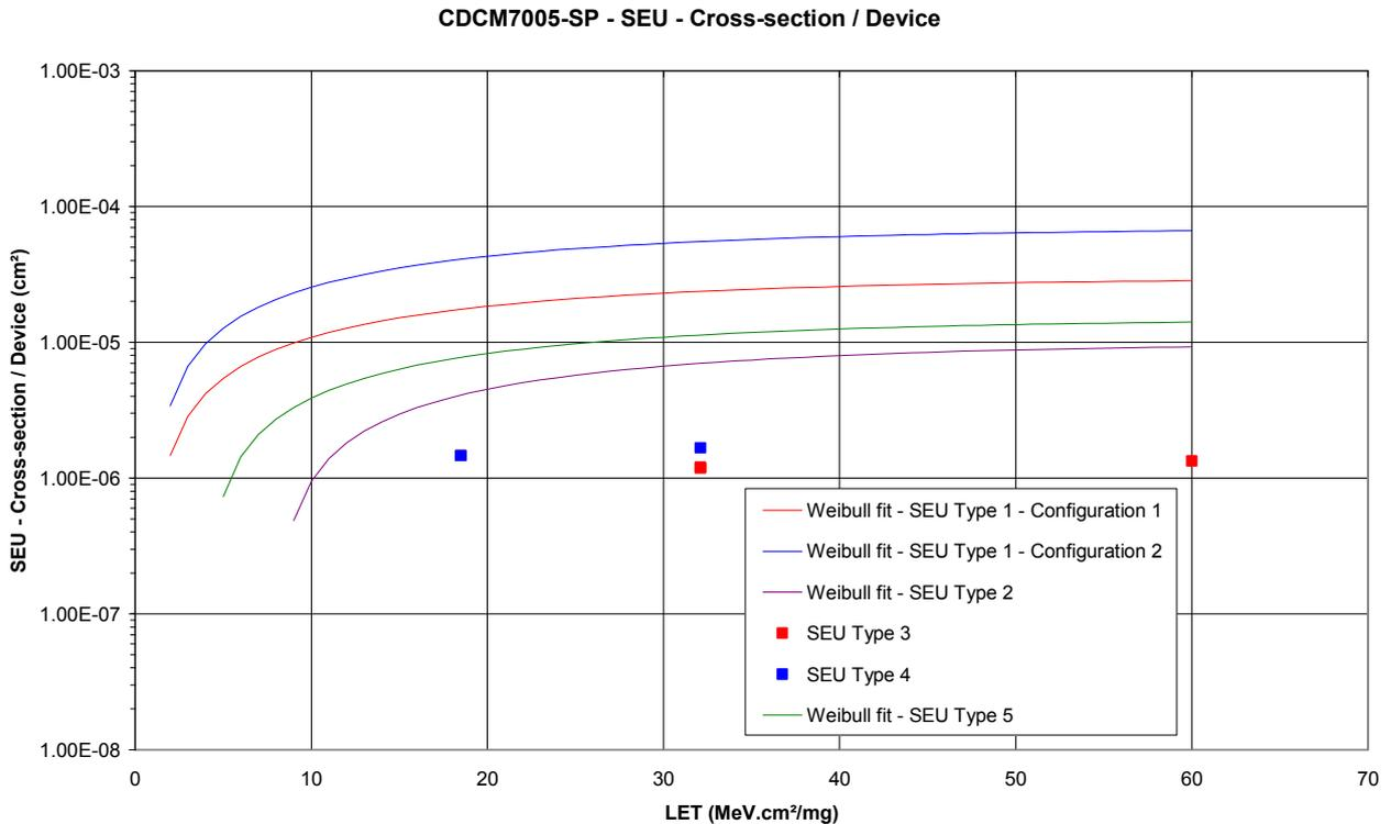
Figure 10 - SEU cross-sections per device
