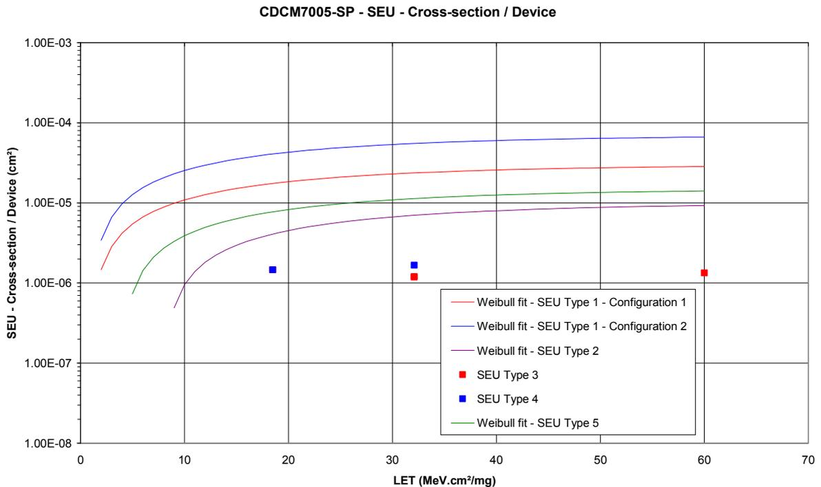
**Figure 1 - SEU cross-section per device**
