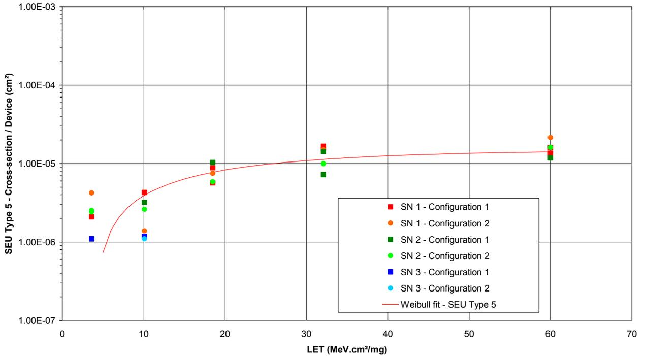
Figure 16 - SEU Type 5 cross-section per device
