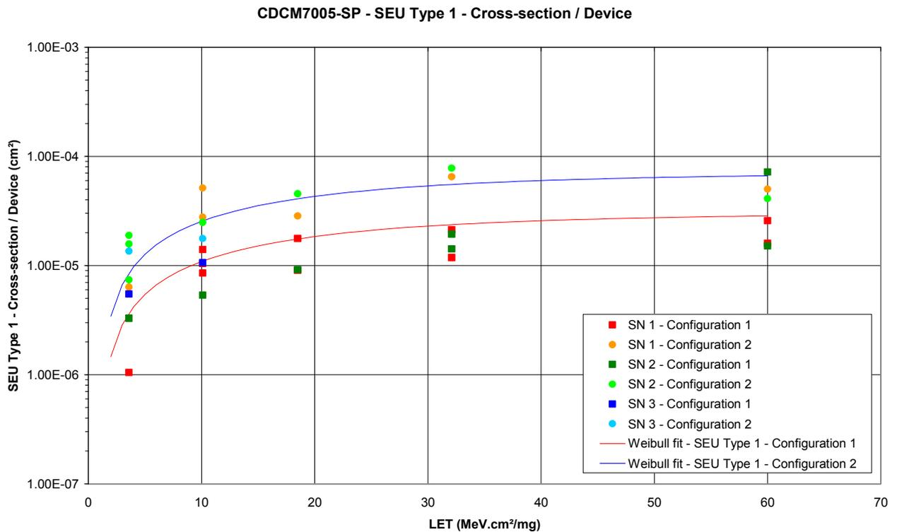
Figure 11 - SEU Type 1 cross-section per device
