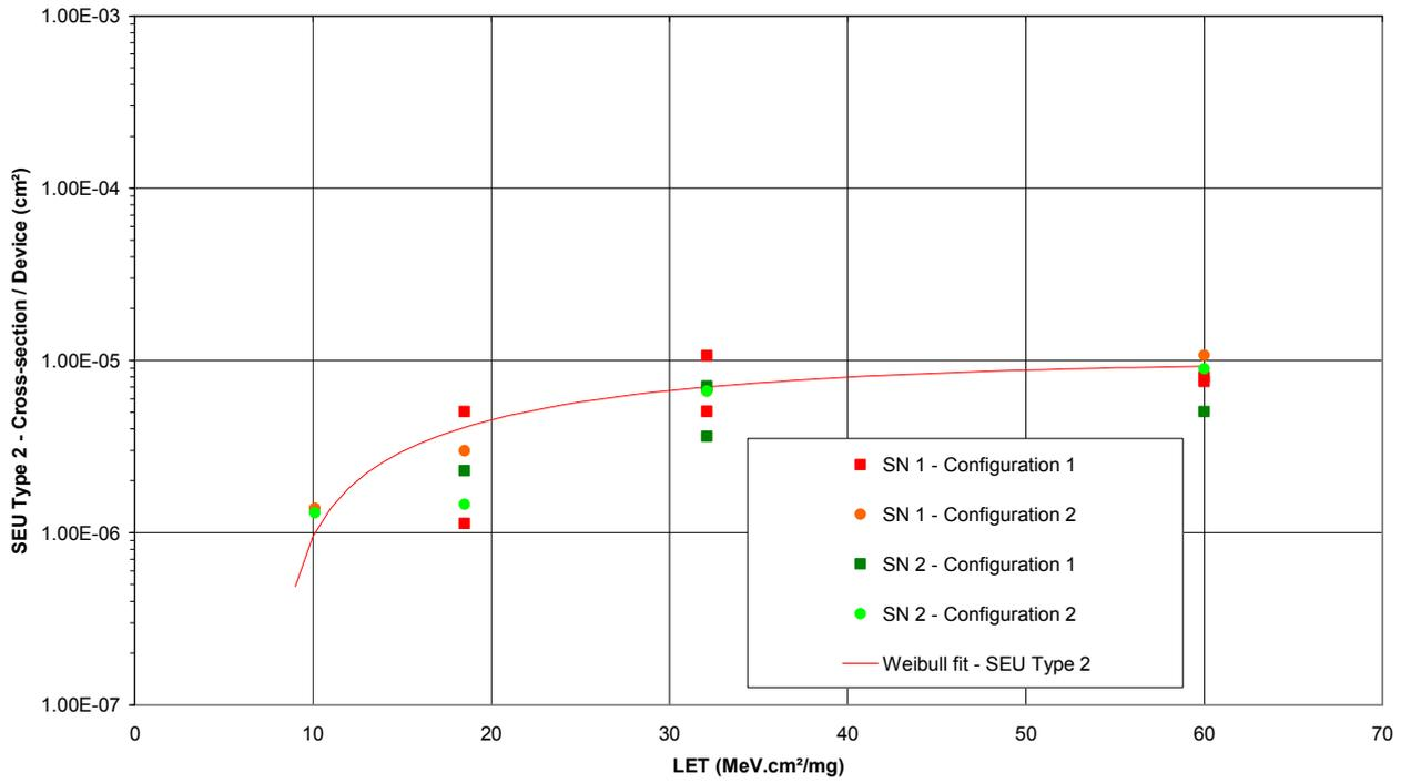
Figure 13 - SEU Type 2 cross-section per device
