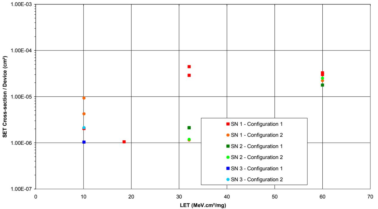
Figure 18 - Vbb - SET cross-section per device
