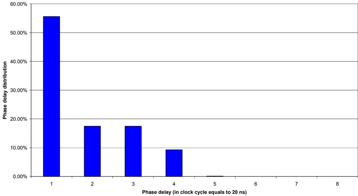
Figure 12 - SEU Type 1 - Phase delay distribution
