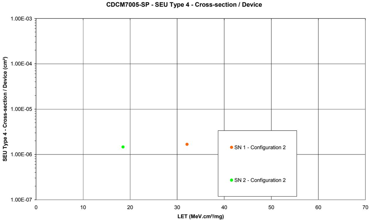
**Figure 15 - SEU Type 4 cross-section per device**
