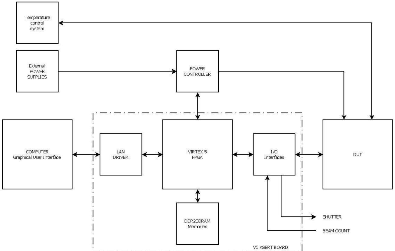
Figure 3 - Heavy ion test set-up
