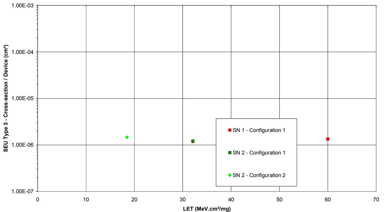
Figure 14 - SEU Type 3 cross-section per device
