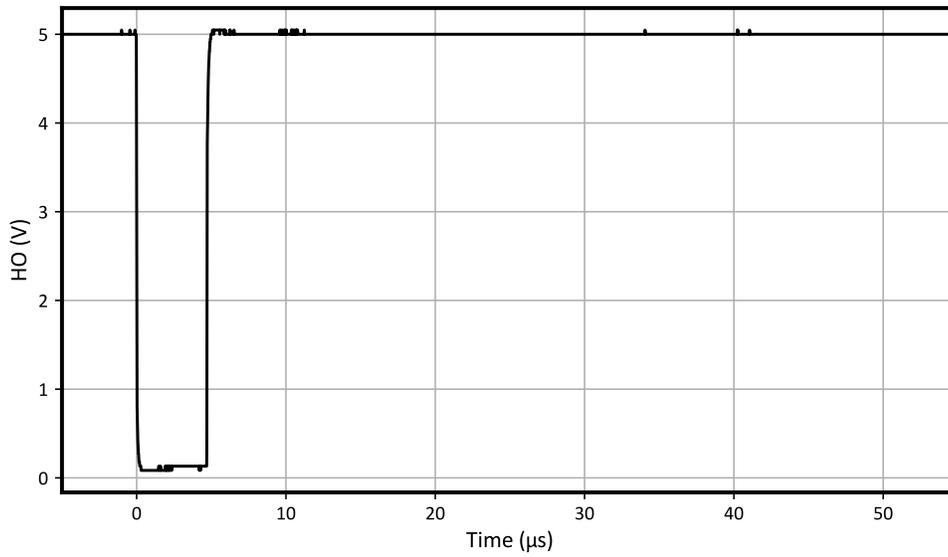
**Figure 8-4. HO SET Run 25 (IIM-Disabled Mode, EN/HI = 5V)**
