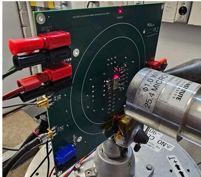
**Figure 4-1. Photograph of the TPS7H60X3-SP Evaluation Board in Front of the Heavy-Ion Beam Exit Port at the Texas A&M Cyclotron**
