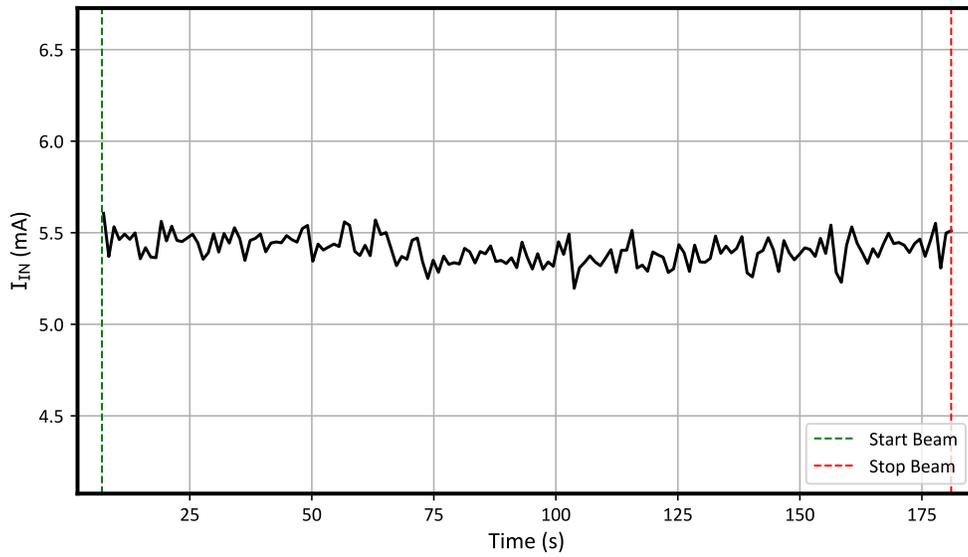
**Figure 7-12. SEB On Run 21 (IIM-Disabled Mode, PWM/LI = 14V)**
