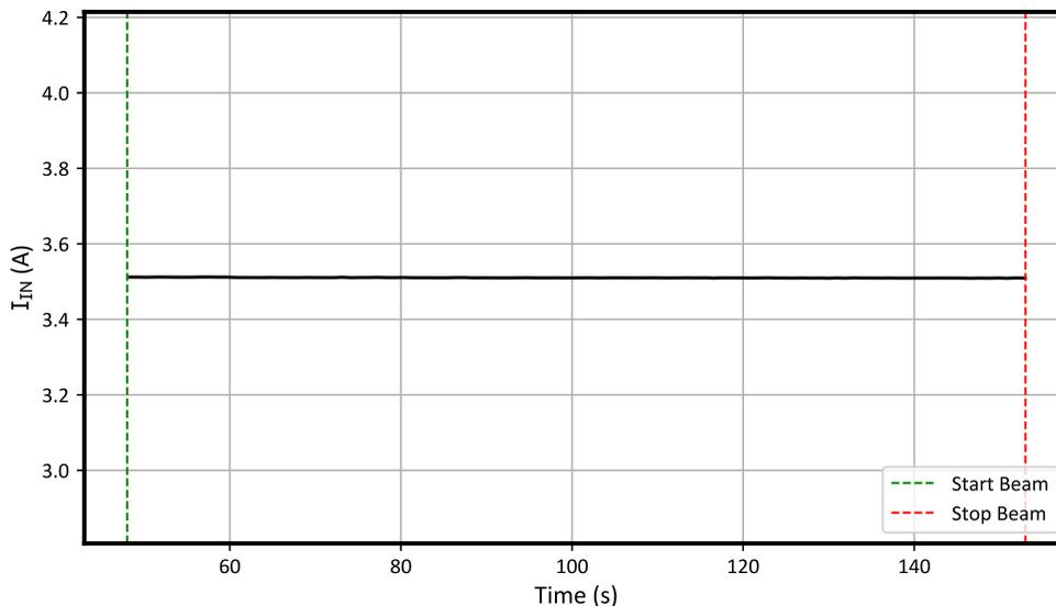
**Figure 7-1. Current vs Time for Run # 1 of the TPS7H2211-SEP at T = 125°C**
