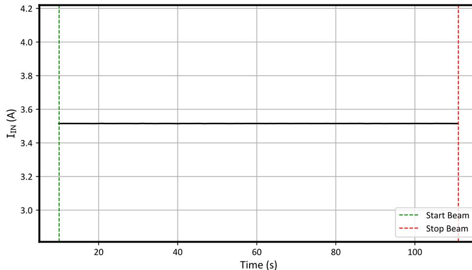
**Figure 7-2. Current vs Time for Run # 4 (Enabled) for the TPS7H2211-SEP at T = 25°C**
