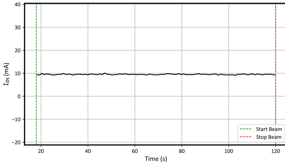
**Figure 7-3. Current vs Time for Run # 5 (Disabled) for the TPS7H2211-SEP at T = 25°C**
