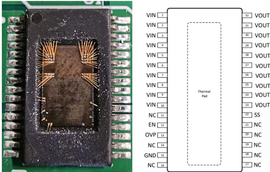
**Figure 3-1. Photograph of Delidded TPS7H2211-SEP (Left) and Pin Out Diagram (Right)**
