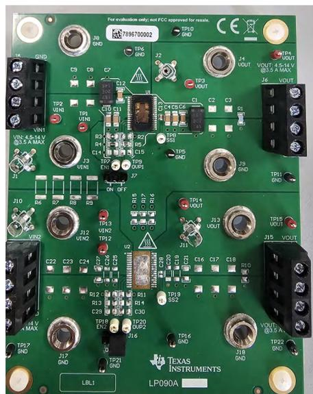
**Figure 3-2. TPS7H2211-SEP Board Top View**
