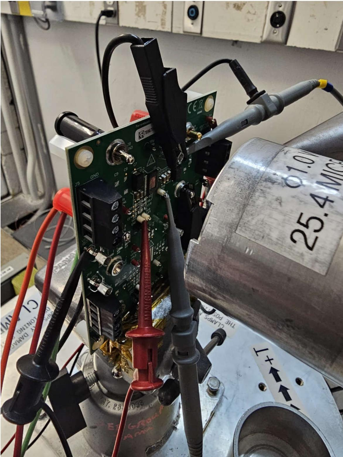
**Figure 4-1. Photograph of the TPS7H2211-SEP Evaluation Board Mounted in Front of the Heavy-Ion Beam Exit Port at the Texas A&M Cyclotron**
