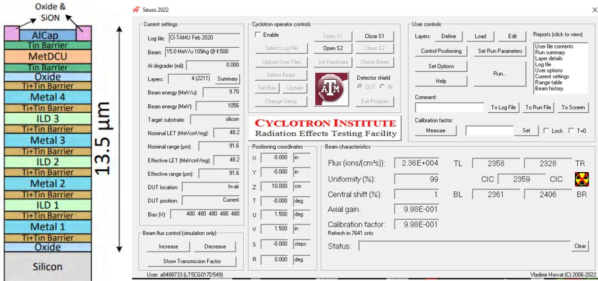
**Figure 5-1. Generalized Cross-Section of the LBC7 Technology BEOL Stack on the TPS7H2211-SEP (Left) and SEUSS 2020 Application Used to Determine Key Ion Parameters (Right)**
