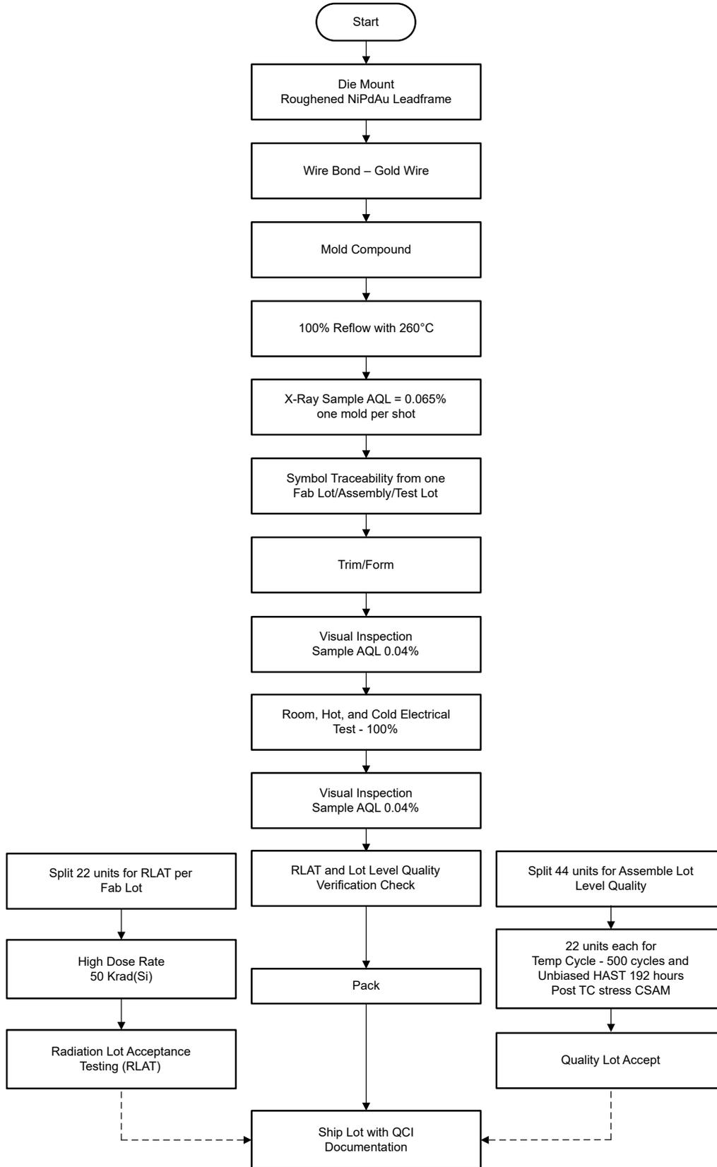
**Figure 2-1. TPS7H500x-SEP Space Enhanced Plastic Production Flow Chart**
